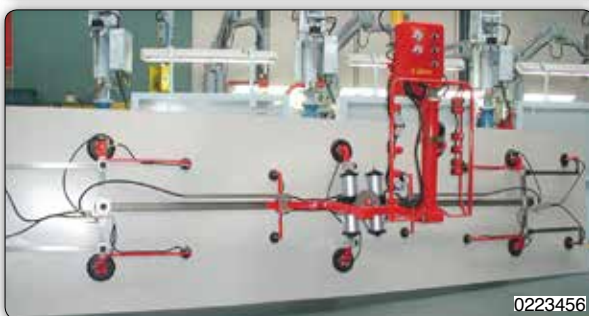
Partner manipulator, overhead trolley mounted with motorised pneumatic drive, fitted with adjustable suction cups tooling for handling and inclination of panels of big dimensions.
