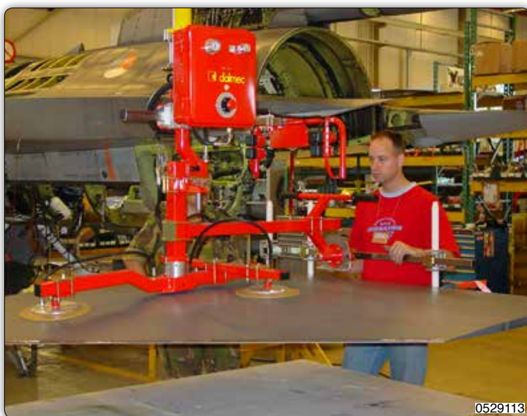
Partner manipulator, column mounted, fitted with adjustable suction cups tooling for handling panels.
