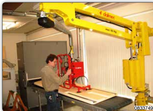
Manipulator with suction tooling for picking plastic panels.
