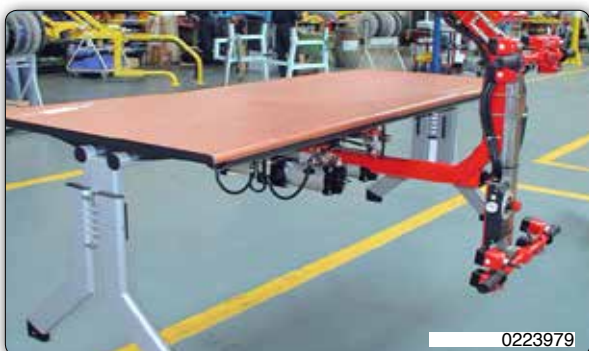
Vacuum suction systems and pneumatic or manual inclination/rotation for handling different types of products.
