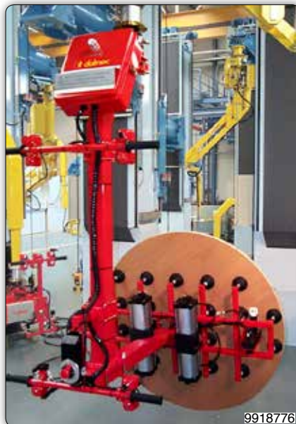
Suction cups tooling for handling and 180° pneumatic rotation of wooden panels.
