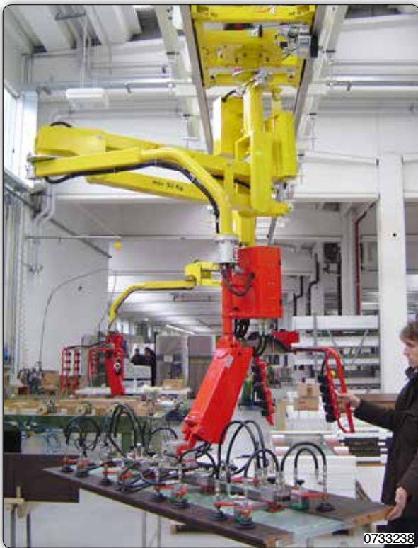
Partner manipulator, overhead trolley mounted, equipped with a suction system for picking sheets of stainless steel, picking them level from a pallet, moving them and depositing the same on another adjacent pallet. The servo-assisted inclination allows the operator to make a visual inspection of the sheet.
