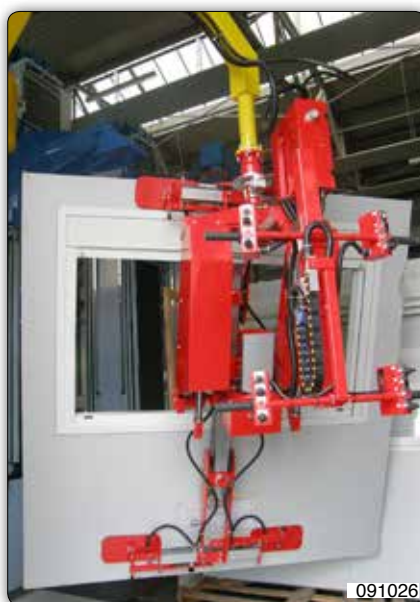
Suction tooling with centerings for handling and inclination of special panels.
