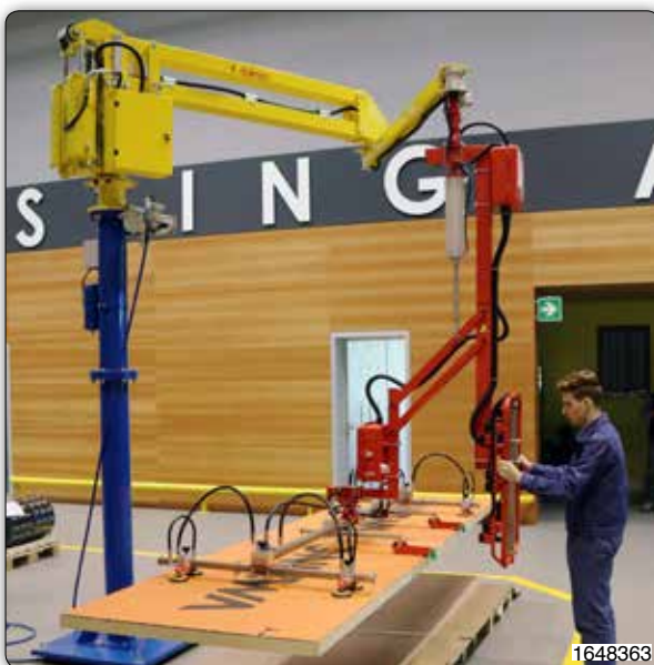
Partner manipulator, column mounted version, equipped with suction cups tooling for the handling of panels. The position of each suction cup may be adjusted manually.
