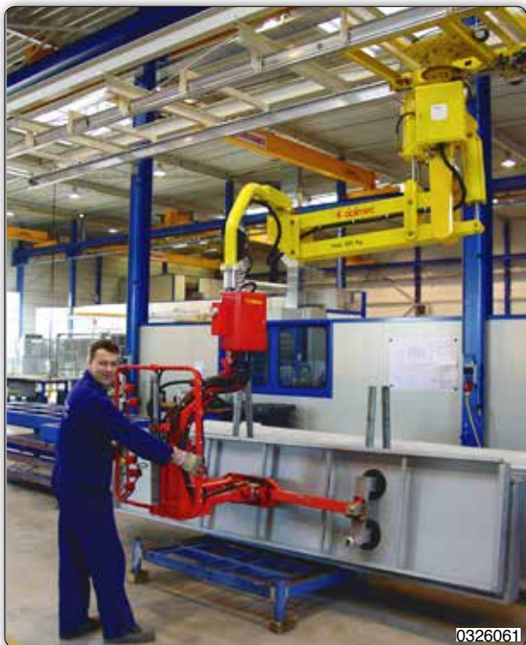
Partner manipulator, overhead trolley mounted with motorised pneumatic drive, fitted with adjustable suction cups tooling for handling and inclination of panels of big dimensions.
