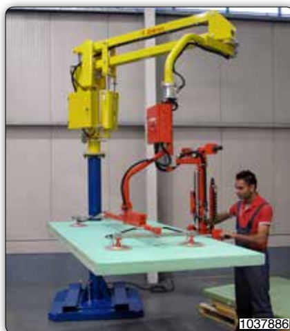
Manipulator with suction tooling for gripping insulating boards.
