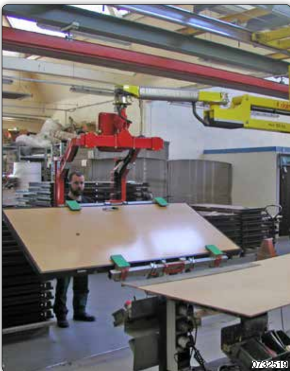
Partner manipulator, column mounted, fitted with two self-centering pairs of grippers, for picking reinforced doors and then rotating them through 180°.
