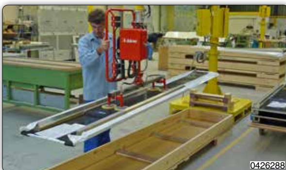
Vacuum suction systems and pneumatic or manual inclination/rotation for handling different types of products.
