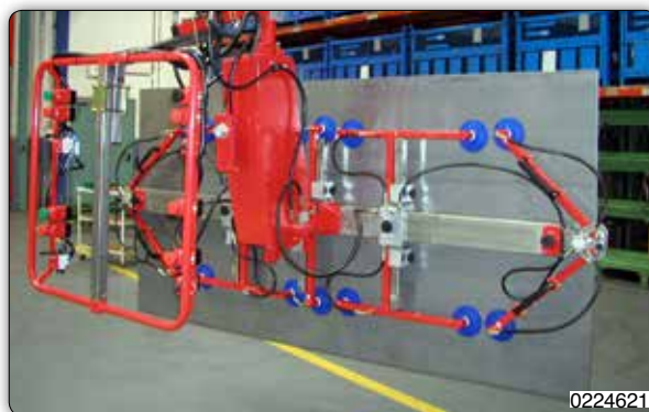
Manipulator with suction tooling for picking plastic panels.
