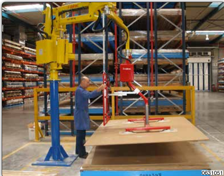
Partner manipulator, column mounted, fitted with suction head for picking a panel from a pallet and then for placing it onto a framing machine following shaving.
