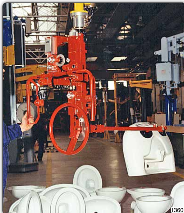
Manipulator with interchangeable suction cups tooling for gripping and handling of sanitary with manual rotation.
