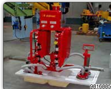
Manipulator with adjustable suction cups tooling (Venturi) for handling and inclination of sinks.
