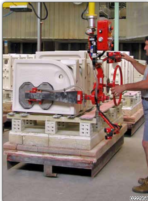
Partner manipulator, fixed overhead, with suction cups tooling (Venturi) for gripping and manual rotation of shower plates.
