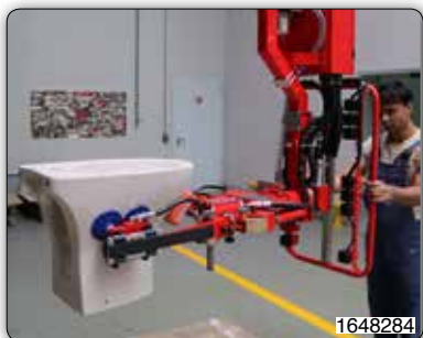
Adjustable forks tooling for handling WC.
