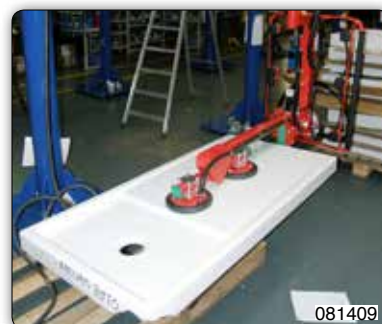
Manipulator with suction cups tooling (Venturi) for gripping shower plates.
