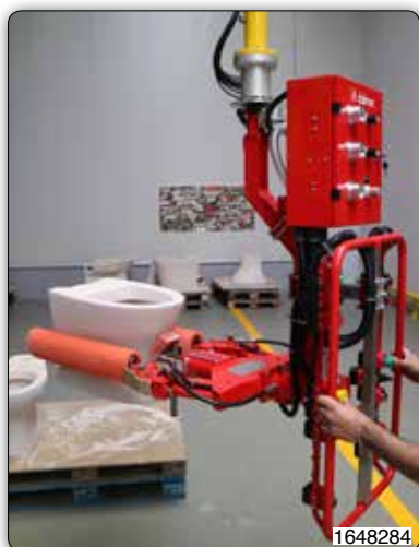
Tooling with adjustable forks covered with sponge rubber for the handling of wc.
