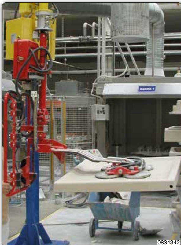
Partner manipulator, column mounted, equipped with suction cups tooling (Venturi) for gripping and manual rotation of raw shower plates.
