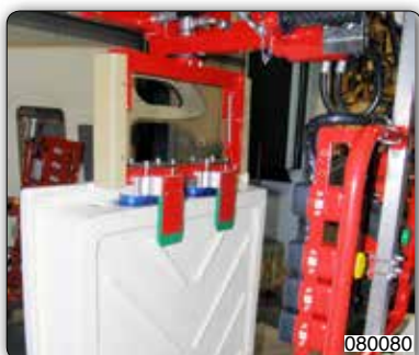
Manipulator with pneumatic tooling for gripping and rotation of shower plates.
