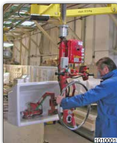
Manipulator with suction cups tooling (Venturi) for gripping and rotation of sinks.
