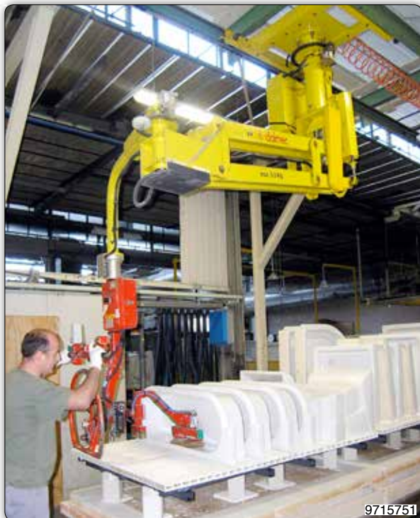
Partner Manipulator, overhead trolley mounted, with interchangeable suction cups tooling for gripping and handling sinks having different dimensions.
