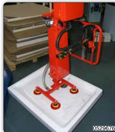
Manipulator with suction cups tooling (Venturi) for gripping shower plates.
