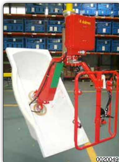
Suction cups manipulator (Venturi) for gripping and inclination of bathtubs.
