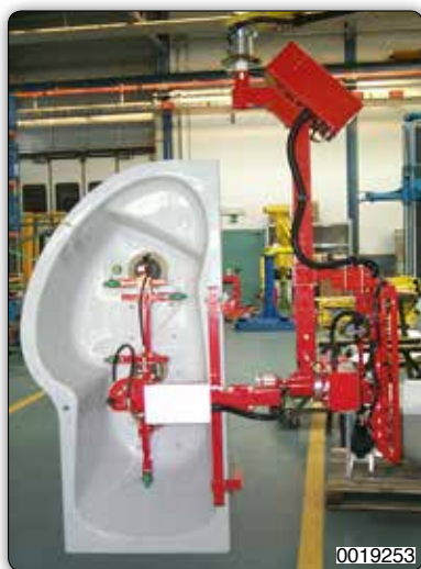
Suction cups (Venturi) manipulator for gripping and rotation of bathtubs.
