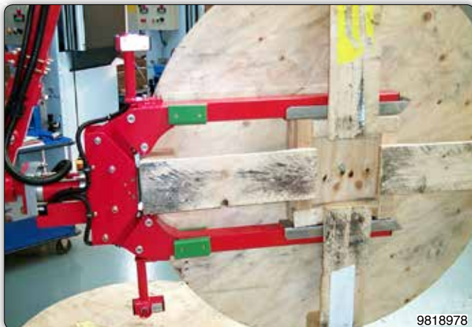
Manipulator with jaws tooling and manual rotation of particular pallets.
