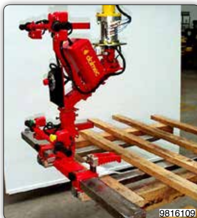
Adjustable forks tooling with block device.
