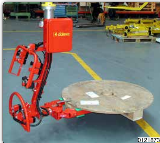
Manipulator with jaws tooling and pneumatic rotation of particular pallets.
