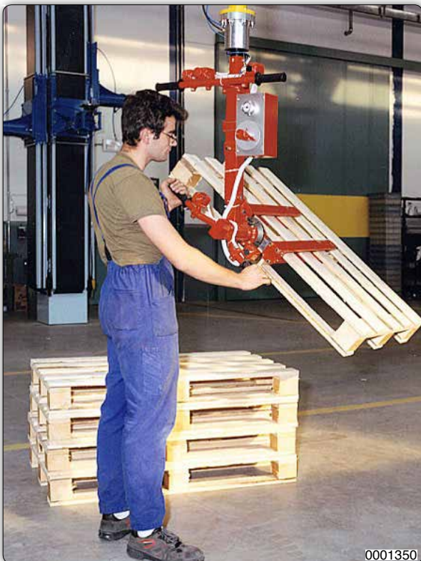
Manipulator with forks type tooling with 180° manual rotation for gripping and overturning pallets.
