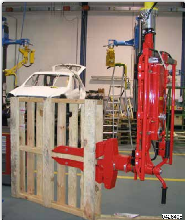
Manipulator with pneumatic tooling with manual of the pallet.
