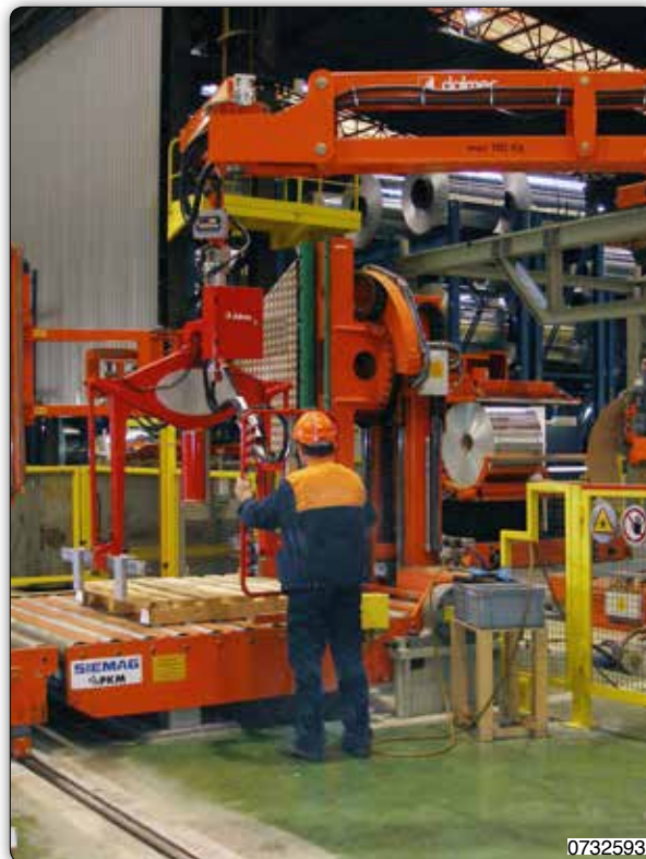
Partner Manipulator, column mounted version, equipped with jaws tooling for gripping pallets.
