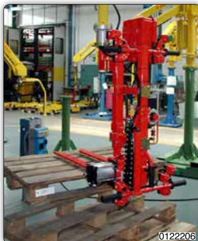
Adjustable forks tooling with pneumatic rotation of the load and telescopic controls.
