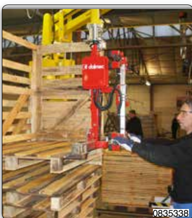
Forks tooling with manual rotation of the load.
