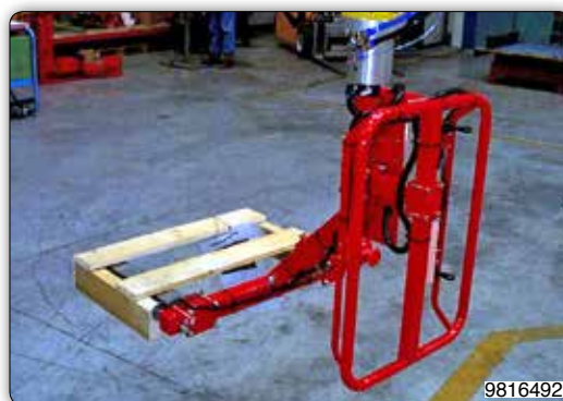
Manipulator with forks type tooling and part presence sensor for handling pallets.
