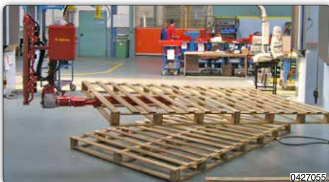
Manipulator with jaws type tooling and manual rotation of particular pallets.
