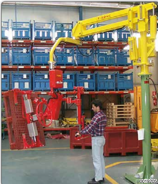
Partner Manipulator, column mounted version, equipped with jaws tooling for gripping, pneumatic inclination and manual rotation of plastic pallets.
