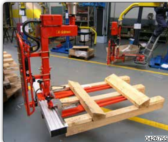
Manipulator with jaws type tooling with manual rotation of the pallet.
