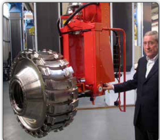
Manipulator with equipment for loading and unloading of aircraft turbines components, with pneumatic inclination.
