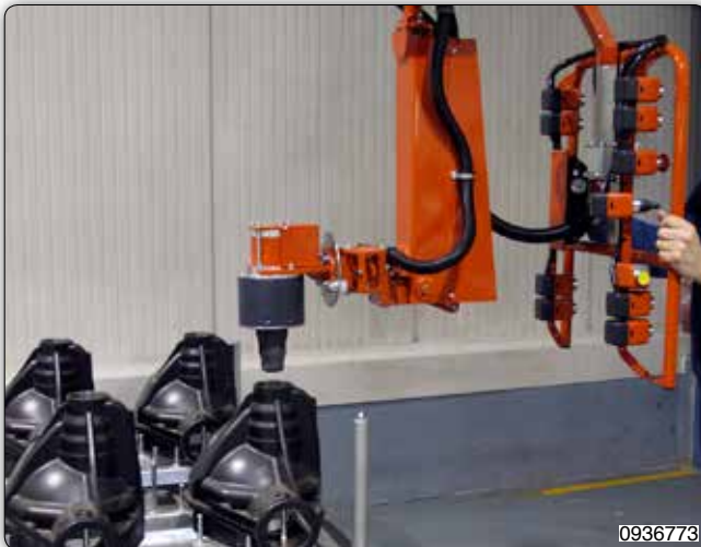
Partner manipulator, column mounted provided with pneumatic pincer to handle with servo-assisted inclination, gearbox casings to be transported to the die-stamping machine.
