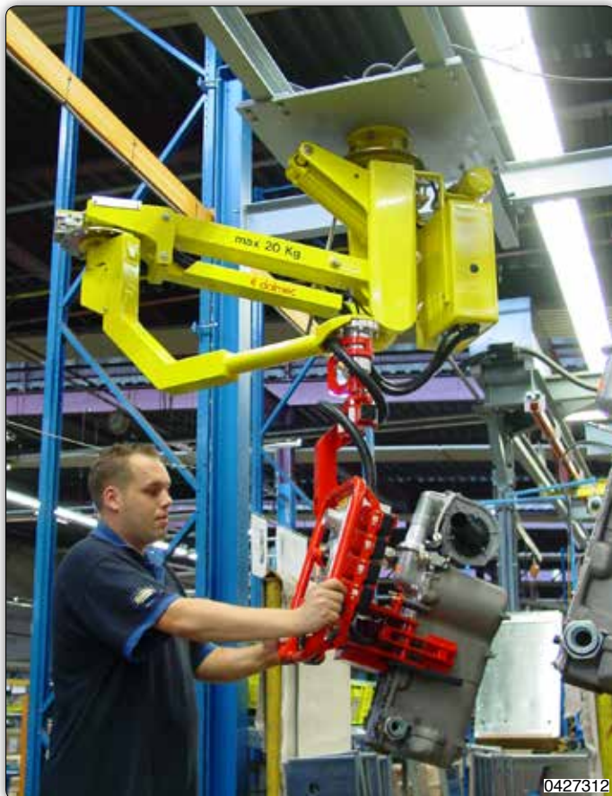
MIS type Micropartner Manipulator, overhead trolley mounted, used for the handling of parts of boilers.
