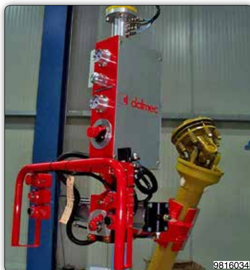
Manipulator with pneumatic gripper for taking and rotating transmission shafts.
