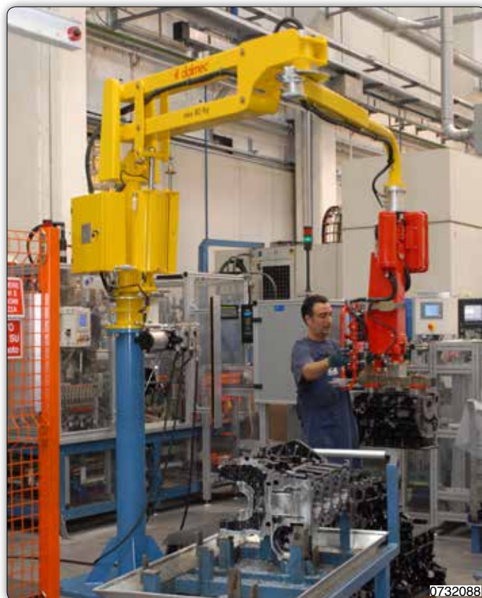
Partner manipulator, column mounted, used to handle crankcases.
