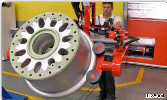
MIS Micropartner manipulator, overhead trolley mounted, with pneumatic tooling for the picking and manual inclination of hubs for use on a machining centre.
