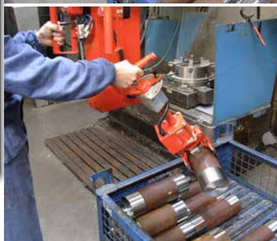
Manipulator with pneumatic gripping tool for picking and 90° pneumatic inclination of cylinders.
