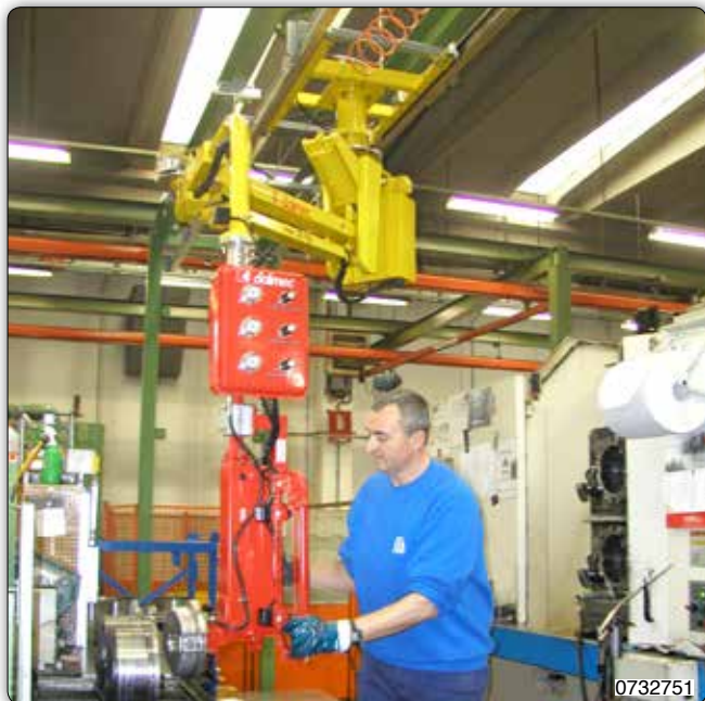
MIS Micropartner manipulator, overhead trolley mounted, with pneumatic tooling for the picking and manual inclination of hubs for use on a machining centre.
