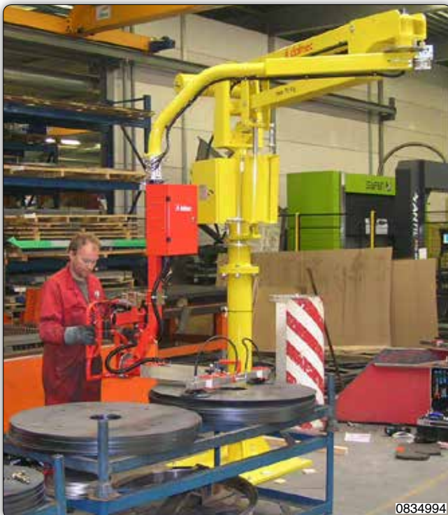
Partner manipulator, column mounted version, with adjustable suction cups tooling for picking sheets.
