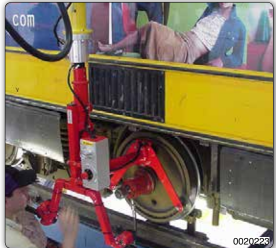
Manipulator with jaws tooling for gripping of railway carriage wheels and their positioning on the carriage.
