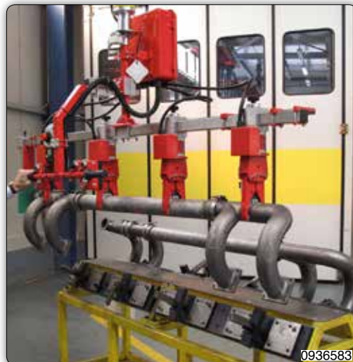
Manipulator equipped with a tooling made up of four adjustable gripping heads pneumatically operated for the gripping of exhaust manifolds.
