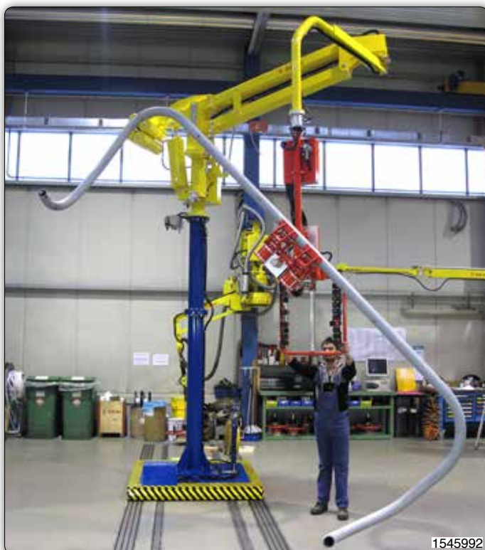
Partner manipulator, column design, with pneumatic gripper equipment, made to move mechanical parts from pallets to a vertical machine tool.
