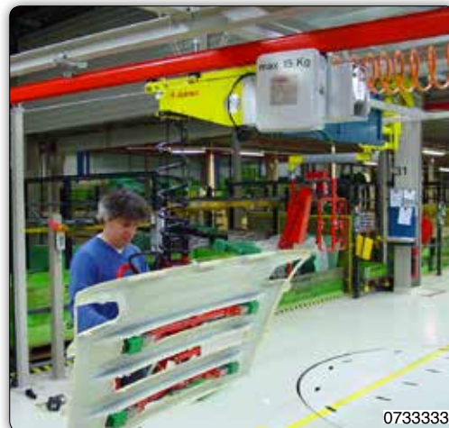
MPS type Minipartner manipulator, overhead trolley mounted running in a rail, equipped with a pneumatic gripper for picking and handling of bodywork parts.
