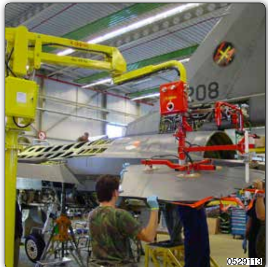
Manipulator with vacuum suction system for moving parts of aircraft wings.
