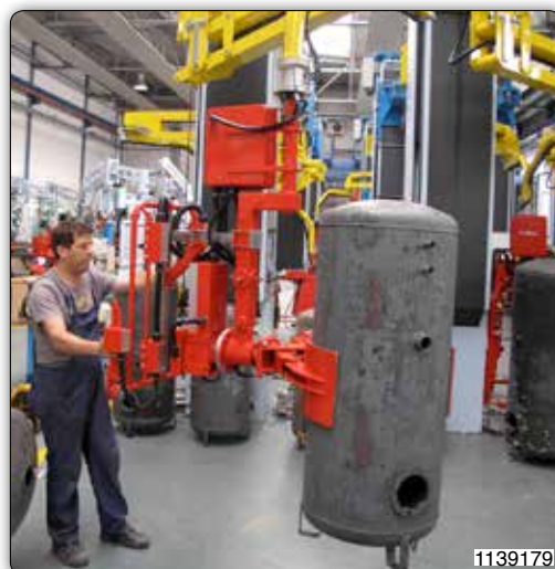
Manipulator with pneumatic gripping tool for picking and 90° pneumatic inclination of cylinders.
