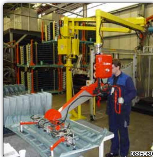
Suction cups gripping system used to handle motor vehicle floor pans from pallets to a support for moulding.
