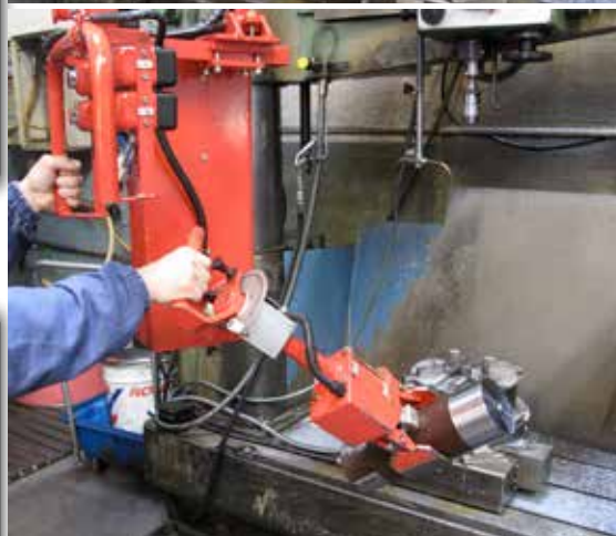
MIS Micropartner manipulator, overhead trolley mounted, with pneumatic tooling for the picking and manual inclination of hubs for use on a machining centre.
