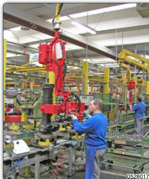
Partner manipulator, column mounted, equipped with pneumatic tooling to pick, handle and, after a 180° rotation, to place axles on a workbench.
