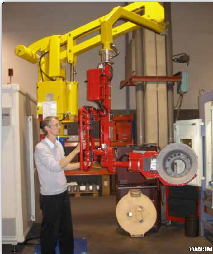
Partner manipulator, column mounted, with pneumatic tooling for picking mechanical components and manually rotating them through 180°, for use on a machining centre.
