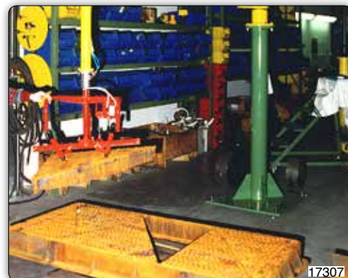
Partner manipulator, column mounted version, equipped with tooling for handling cast-iron covers.
