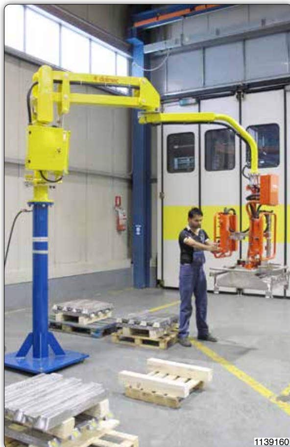
Manipulator with gripping jaws for picking and handling melted ingots.
