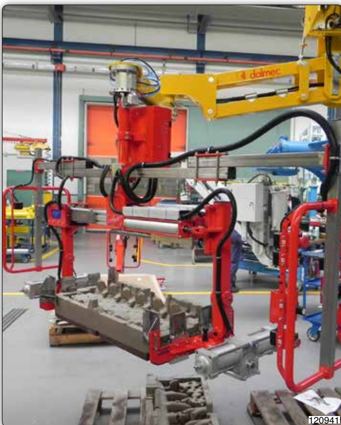
Manipulator with gripper tooling for picking and tipping casting cores.
