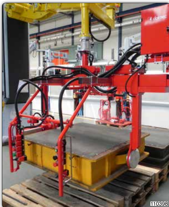
Partner type manipulator, column mounted version, equipped with gripper picking system for moving cores.
