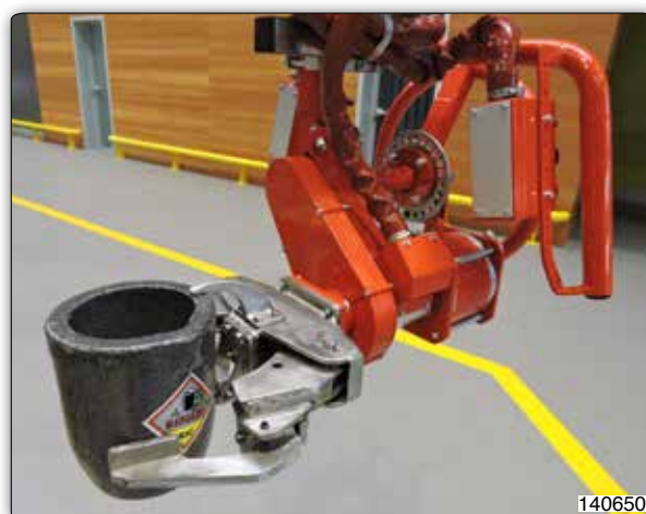
Manipulator with pneumatic gripping jaws for picking and emptying ladles.
