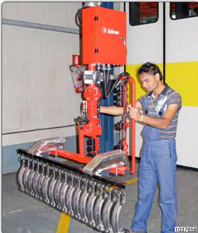
Partner manipulator, column mounted version, with tooling for handling castings.
