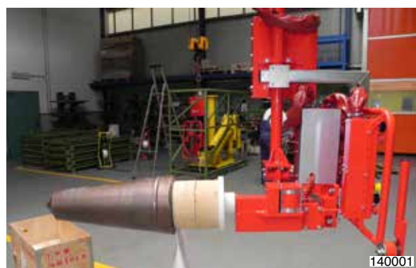
Partner manipulator, overhead trolley mounted version, fitted with fork tooling for handling ladles or crucibles.
