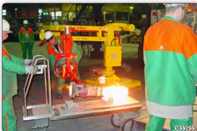
Partner manipulator, column mounted version, equipped with gripping jaws for moving incandescent parts.
