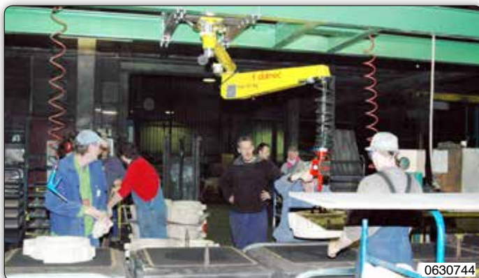
PVS type Posivel manipulator, overhead trolley mounted version, equipped with gripper picking system for moving core boxes.
