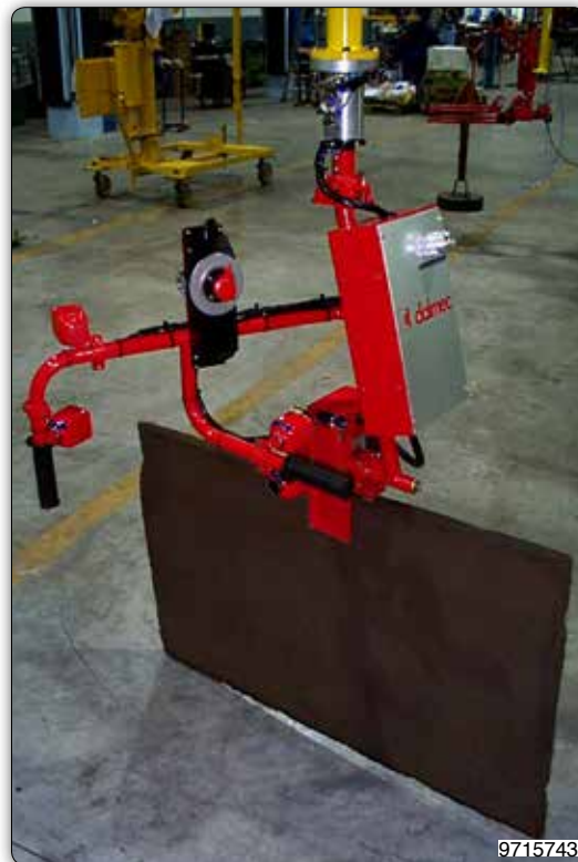
Manipulator equipped with gripper tooling for handling refractory plates.
