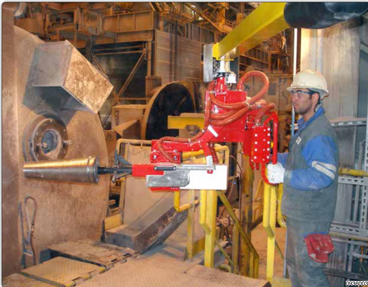
Partner type manipulator, column mounted version, equipped with pneumatic gripper for castings.
