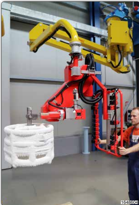
Partner manipulator, overhead trolley mounted version, with pneumatic jaws for picking casting dies.
