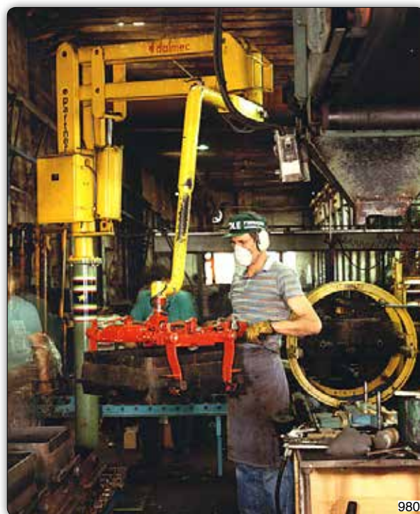
Partner type manipulator, column mounted version, equipped with gripper picking system for moving cores.
