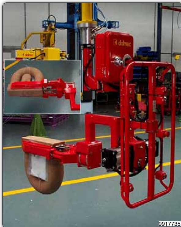
Manipulator equipped with a pneumatic gripper tooling for picking and tipping casting dies.
