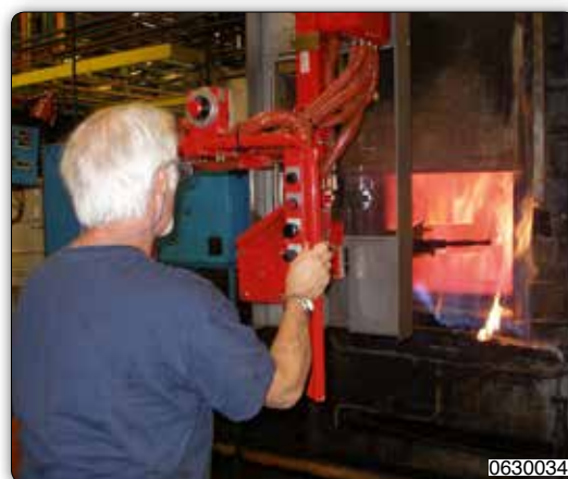
Partner manipulator, column mounted version, equipped with gripping jaws for moving incandescent parts.
