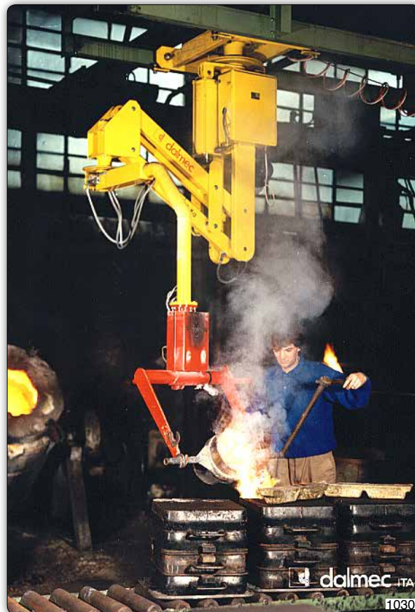
Partner manipulator, overhead trolley mounted version, fitted with fork tooling for handling ladles or crucibles.
