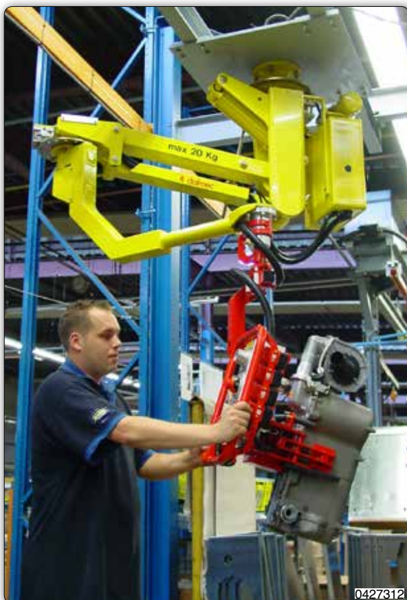
Manipulator equipped with a pneumatic gripper for picking and handling aluminium parts.
