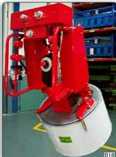
Manipulator with ring-shaped suction cup for gripping and 90° pneumatic inclination of reels.
