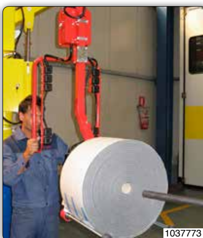
Manipulator equipped with gripper tooling, for handling reels about their external diameter, with pneumatically assisted rotation through \pm 90^\circ .
