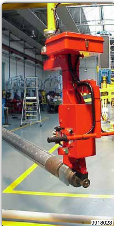
Partner manipulators, column mounted, complete with pneumatic gripper for picking and handling reel-carrier shafts.
