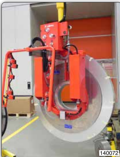
Manipulator with suction cup tooling (Venturi) for gripping and 90° pneumatic inclination of reels. The suction cup is ring shaped.
