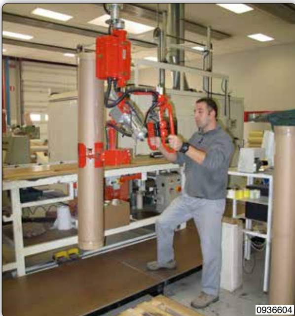
Partner manipulator, column mounted version, with self-centering jaws for the handling of paper reels. The equipment is designed to pick horizontal reels from a winding shaft and then place them vertically to an adjacent pallet. Rotation is actuated pneumatically.
