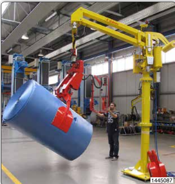
Partner manipulator, column mounted version. The gripper tooling is provided with interchangeable jaws for handling reels about their external diameter with different dimensions and it is equipped with a pneumatic system for the 90° inclination.
