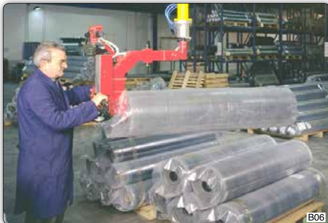
Manipulator with tooling for handling rolls of rubber from a packaging line to a pallet, made up of a pin which is inserted into the core of the roll.
