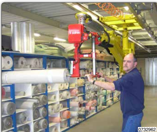
Partner manipulator, overhead trolley mounted version to run in an aluminum tracking system. The tooling is made up of a pin suitable for handling rolls of cloth.
