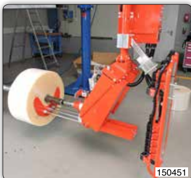
Mandrel gripping system equipped with pusher to facilitate the release of the reel.
