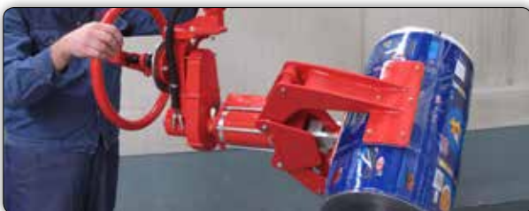
Partner manipulator, column mounted version. The gripper tooling is provided with interchangeable jaws for handling reels about their external diameter with different dimensions and it is equipped with a pneumatic system for the 90° inclination.
