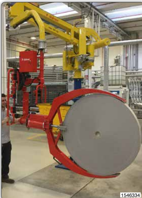
PEC type Partner manipulator, column mounted, with gripper tooling, for handling reels about their external diameter, with 360° manual rotation.
