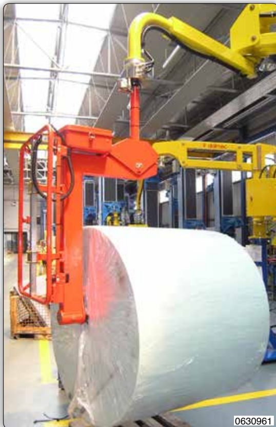
Partner manipulator, column mounted, provided with a gripping tooling with pin for handling big reels.
