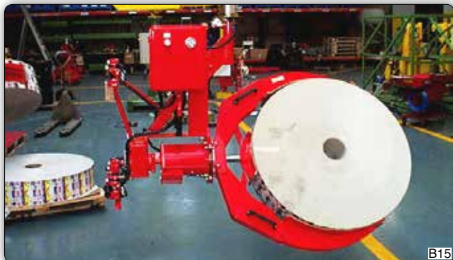
PEC type Partner manipulator, column mounted, with gripper tooling, for handling reels about their external diameter, with 360° manual rotation.
