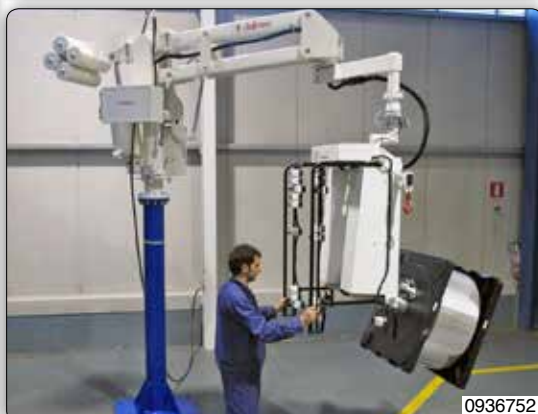
MXC type Maxipartner manipulator, column mounted version. The tooling consists of an expanding mandrel complete with a pneumatic 90° inclination system.
