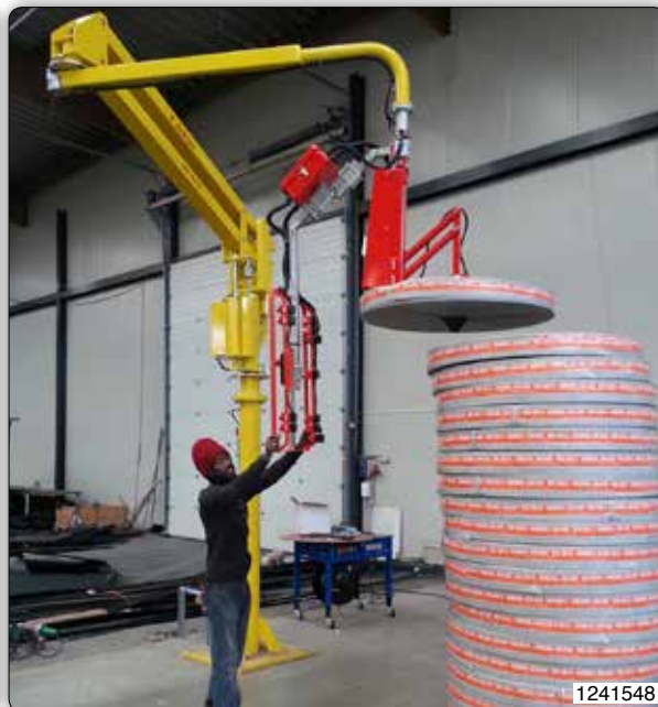
Partner Manipulator, column mounted version, suitable for the handling of reels. The tooling consists of an expanding mandrel mounted on a parallelogram, suitable for gripping the reel in its core. The system enables to increase the vertical lift allowing the stacking of the reels.
