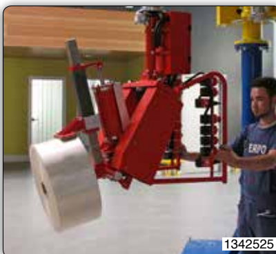
PEC type Partner manipulator, column mounted. The tooling consists of an expanding mandrel and it is equipped with a pneumatic system for 90^\circ inclination and also with an anti-telescoping device.
