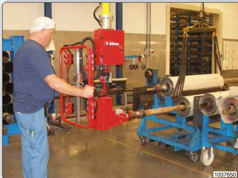
Partner manipulators, column mounted, complete with pneumatic gripper for picking and handling reel-carrier shafts.
