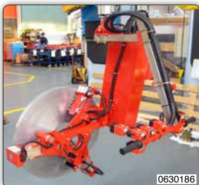
Manipulator equipped with magnets tooling for gripping and 90° inclination of rolls of metallic banding.
