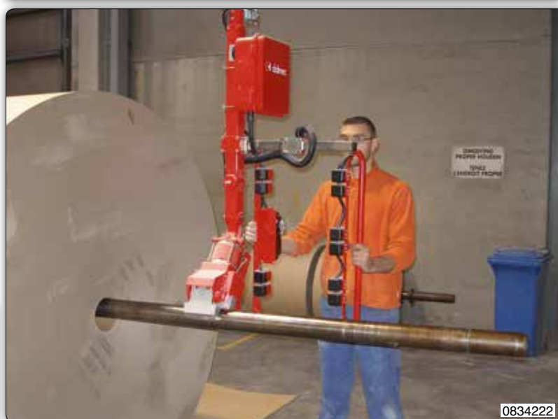
Manipulator equipped with pneumatic gripper for picking and handling carrier shafts.
