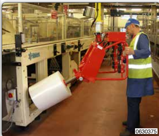
Manipulator with adjustable forks type tooling for handling rolls of plastic film.
