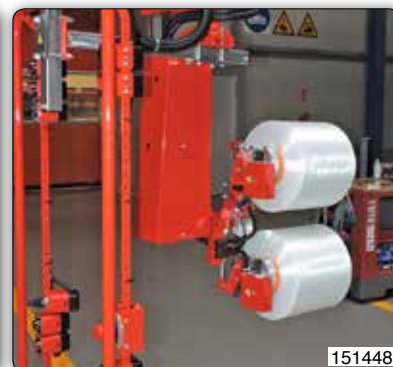
Manipulator equipped with expanders for gripping two spools simultaneously.
