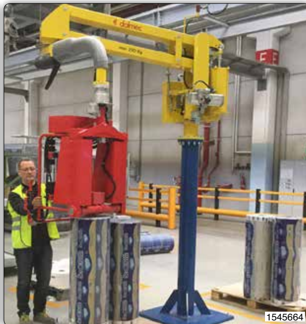
Partner manipulator, column mounted version, fitted with pneumatic mandrel tooling for gripping in the reel's core and 90° inclination. The unit is used for palletizing reels.
