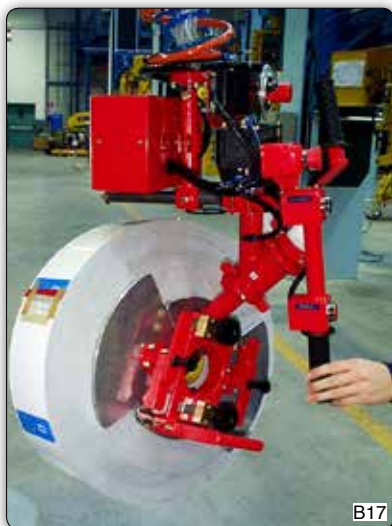
Manipulator with Venturi suction cups tooling for gripping reels, with manual rotation from horizontal to vertical axis.
