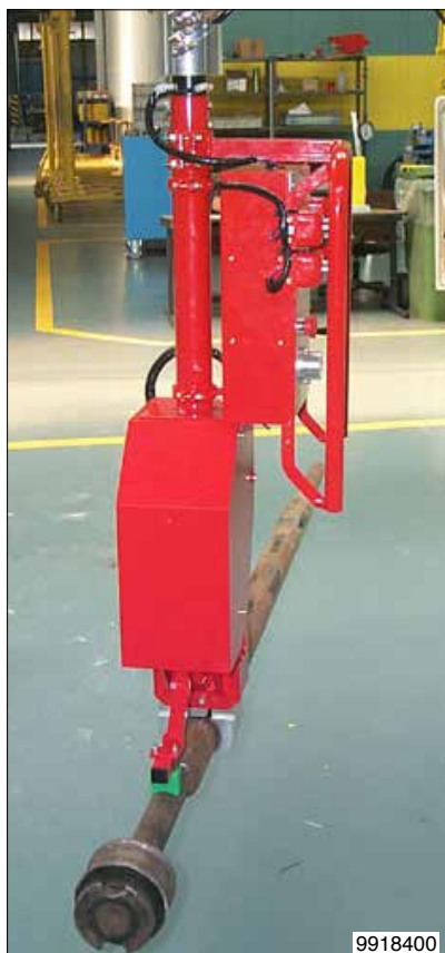
Manipulator equipped with pneumatic gripper for picking and handling carrier shafts.
