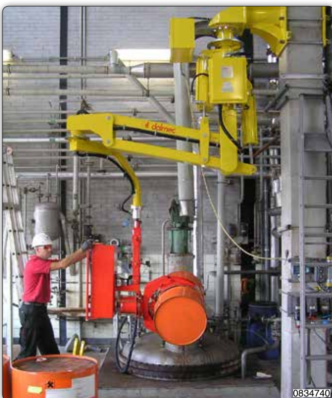
Partner manipulator, fixed overhead, made for picking and emptying drums, weighing up to 400 Kg.
