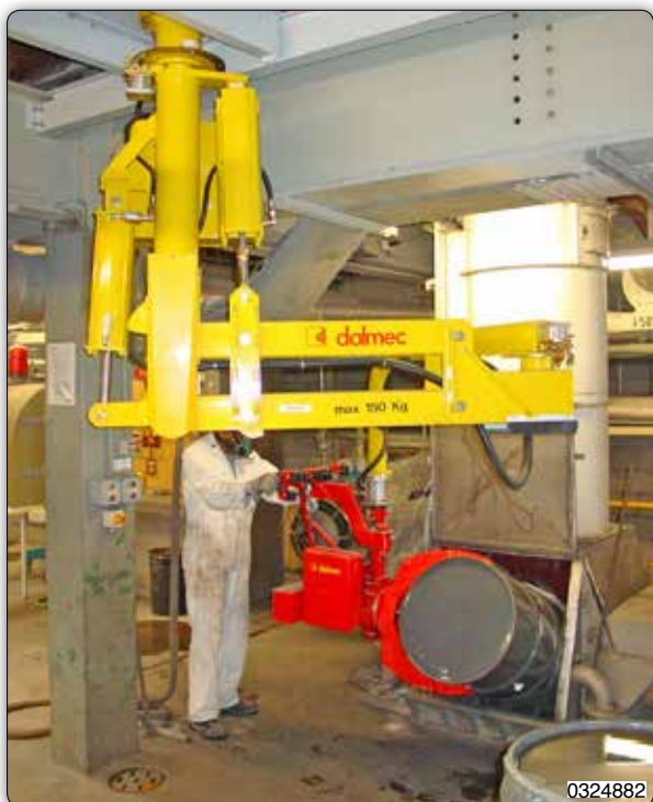
Partner manipulator, fixed overhead version, designed for the picking and emptying of drums.
