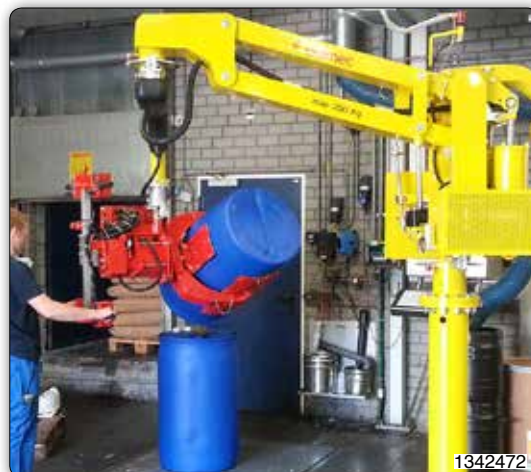
Partner manipulator, column mounted, designed for picking and emptying drums.
