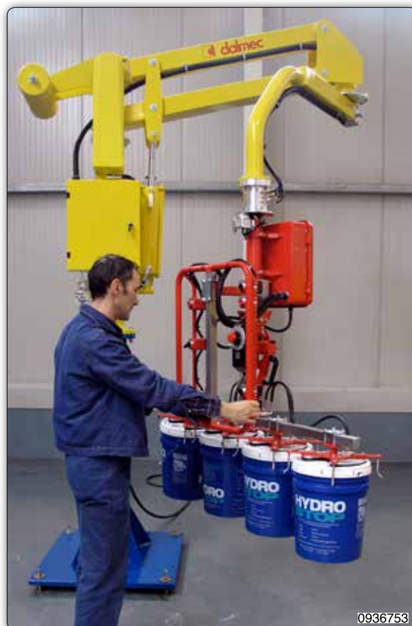
Partner manipulator, column mounted, for handling one or more pairs at once and handling from the packaging line to a pallet.
