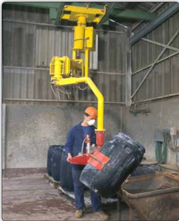
Partner manipulator, overhead trolley mounted version to cover several work stations, for handling and tipping drums.
