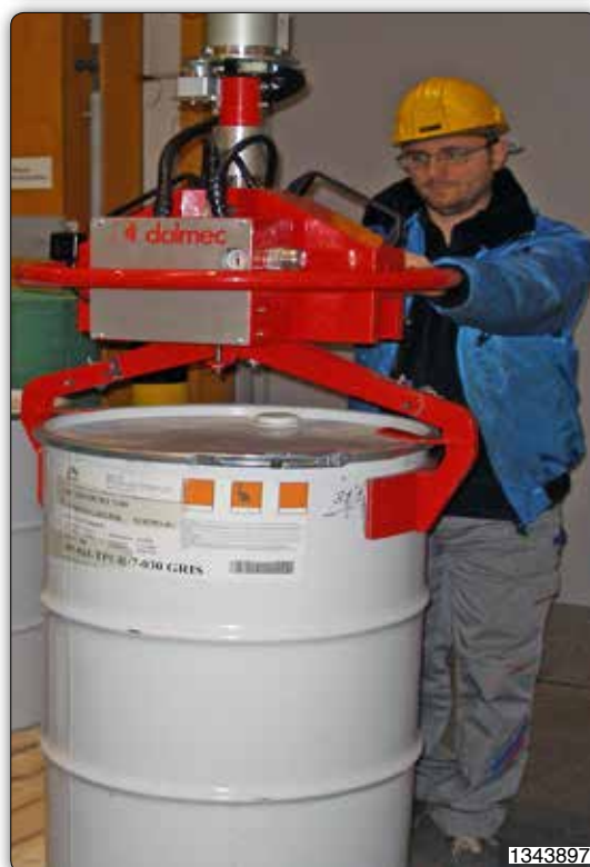
Partner manipulator, column mounted, equipped with tooling for gripping on the drum's rim.
