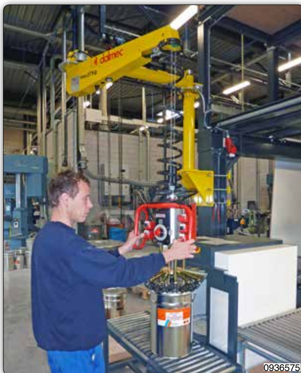
PVC type Posivel manipulator, equipped with pneumatic tooling for closing and gripping pails on the upper edge.
