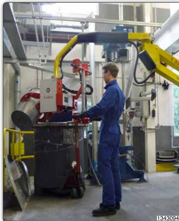
Partner manipulator, column mounted version, designed for picking and emptying drums.
