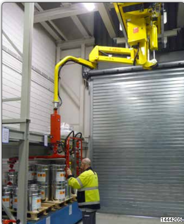
PES type Partner manipulator, overhead trolley mounted version, with a vacuum tooling head, vacuum being generated by Venturi ejector.
