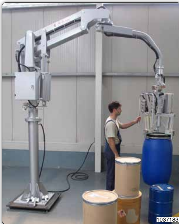
Partner manipulator, column design, equipped for picking and moving drums of varying shape and weight. Interchangeable grippers are available for handling different sizes of drums.
