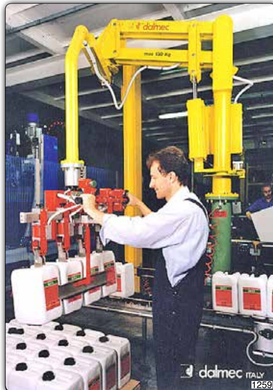
Partner manipulator, column mounted version, equipped with a pneumatic gripper tooling head to handle four canisters at the same time.
