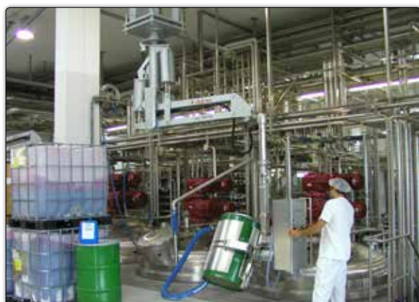
PFF type Posifil manipulator, fixed overhead version for handling metal drums.
