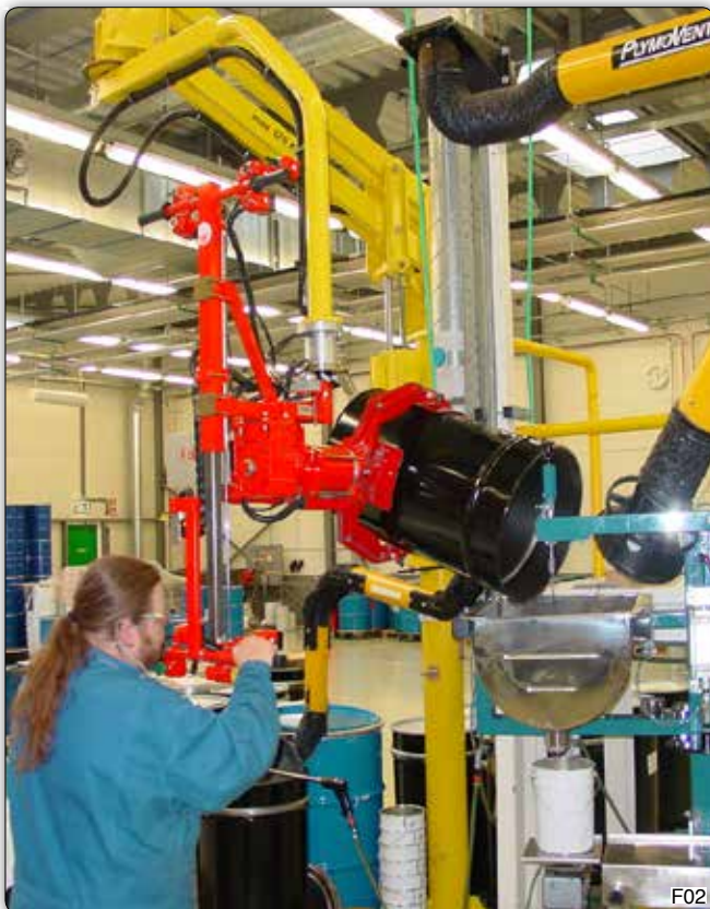
Partner manipulator, column mounted, designed for picking and emptying drums.
