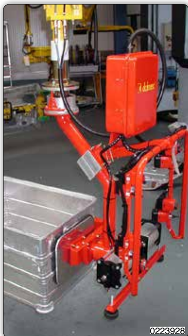
Manipulator with suction cups tooling for handling metallic containers.
