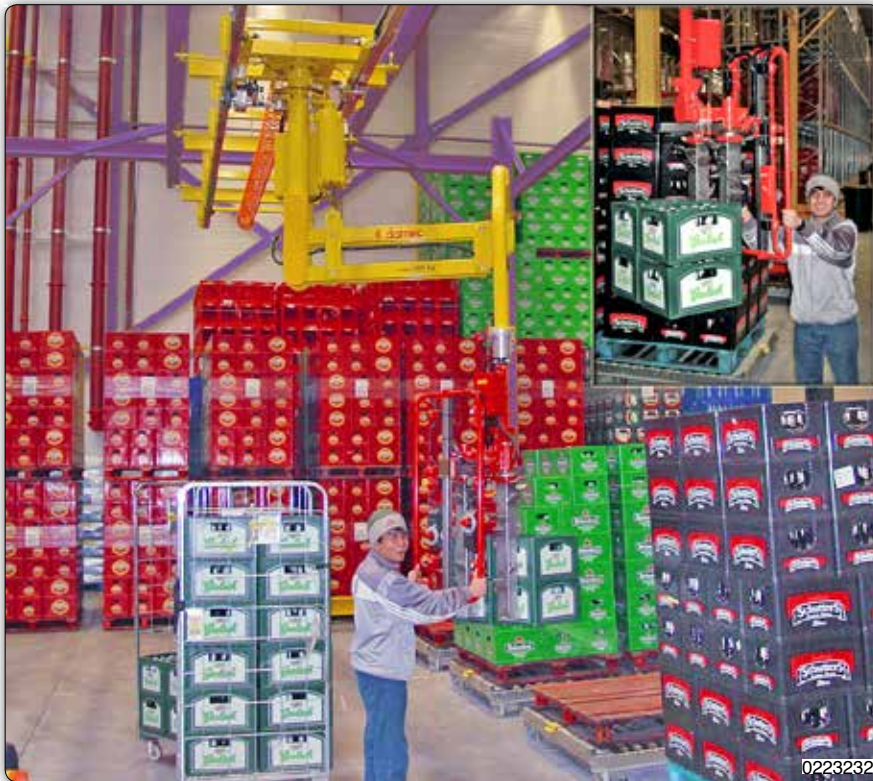
Partner Manipulator overhead trolley mounted version with pneumatic motorization, equipped with multiple adjustable hooks gripping system for handling 1 to 8 beverage crates having different dimensions.
