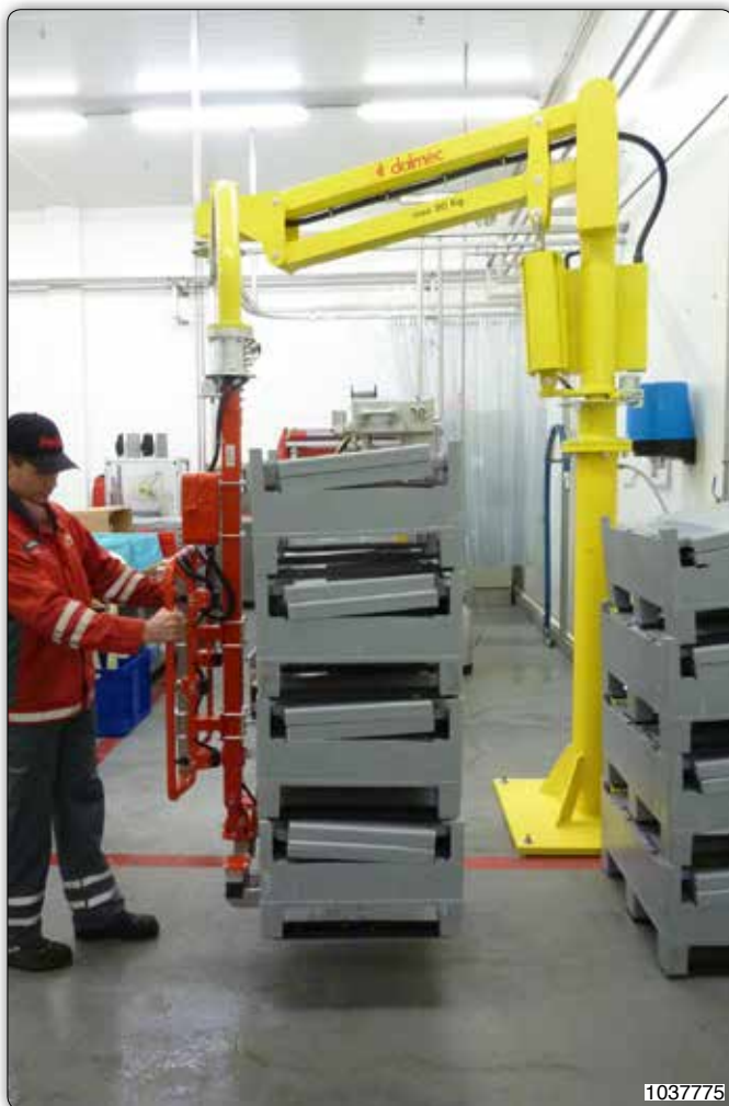
Manipulator with fork type tooling for gripping and handling containers.
