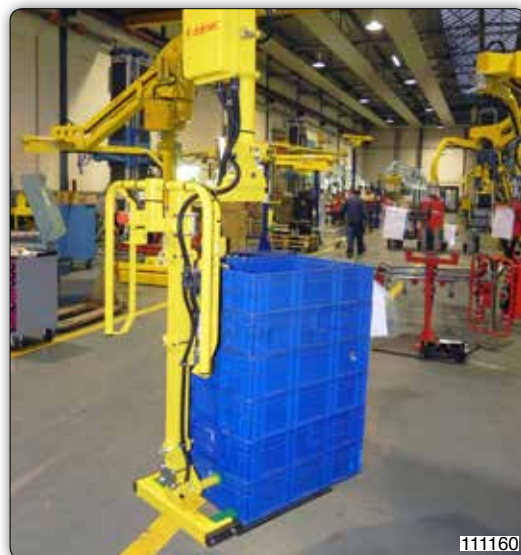
Manipulator with fork type tooling for gripping and handling containers.
