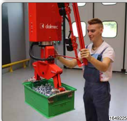
Manipulator with particular pinch jaws tooling for the gripping inside or outside of different types of containers.
