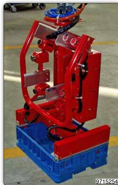
Manipulator with jaws tooling for gripping on the upper edge of the containers.
