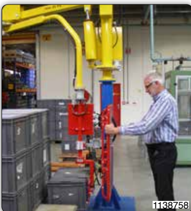
Partner Type balancer, column mounted with pneumatic tooling for gripping, inclination and manual rotation of plastic containers having different dimensions.
