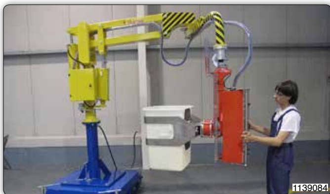
Manipulator with fork type tooling for handling plastic cases.
