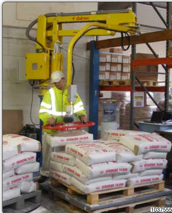
PSC type Partner manipulator, column mounted, equipped with suction head to pick bags from a pallet and to load them to a mixer.
