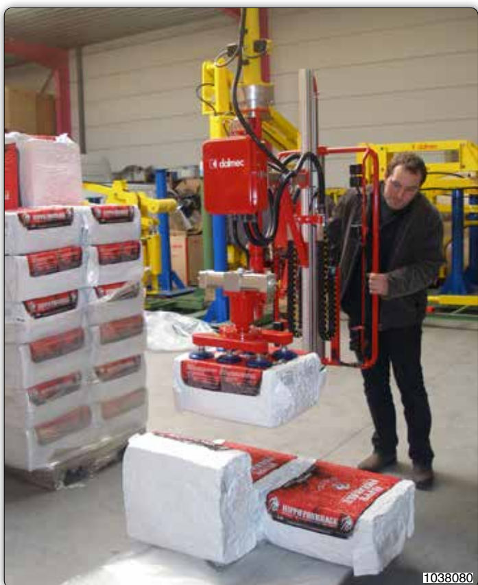
Partner manipulator, column mounted, with suction cups tooling for handling vacuum-packed forage. The tooling is equipped with telescopic controls.
