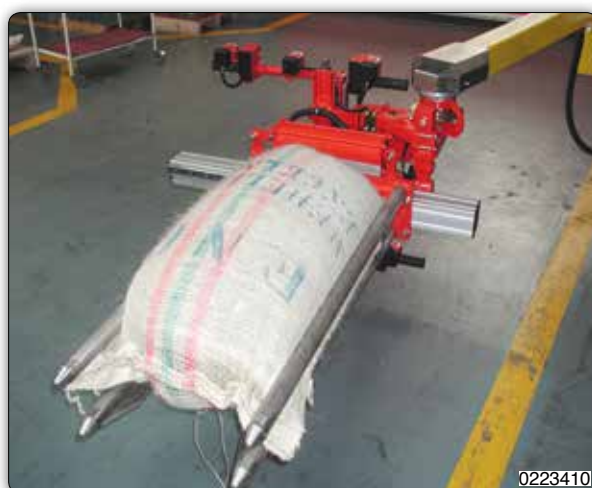
Manipulator with pneumatically actuated gripper picking system.
