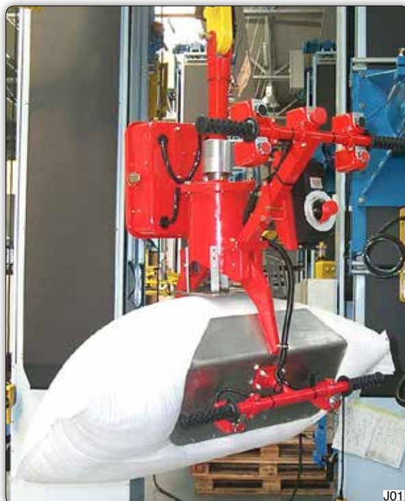
Manipulator with pneumatically actuated gripper picking system.
