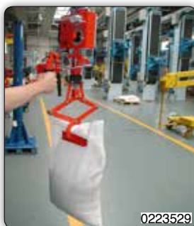
PSC type Partner manipulator, column mounted for palletization/depalletization of bags which are stacked up to about two metres from floor level, fitted with lowered controls.
