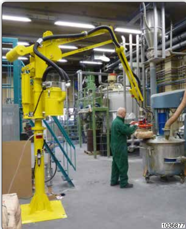
PSC type Partner manipulator, column mounted for palletization/depalletization of bags which are stacked up to about two metres from floor level, fitted with lowered controls.
