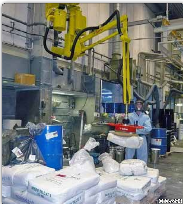
PSS type Partner manipulator, overhead trolley mounted version in Dalmecc track. The operator picks bags from various pallets in the "picking" area and deposits them to a common pallet.
