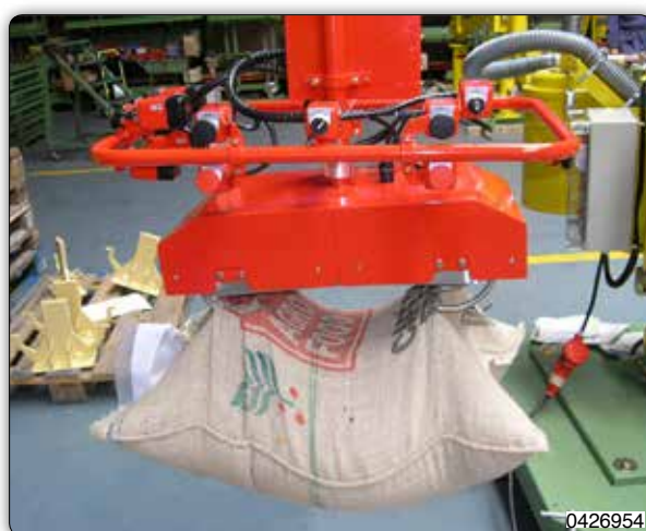
Manipulator with retractable hooks for handling hessian sacks.
