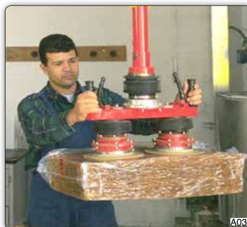
Tooling head for handling rubber bales with independently swivelling suction cups.
