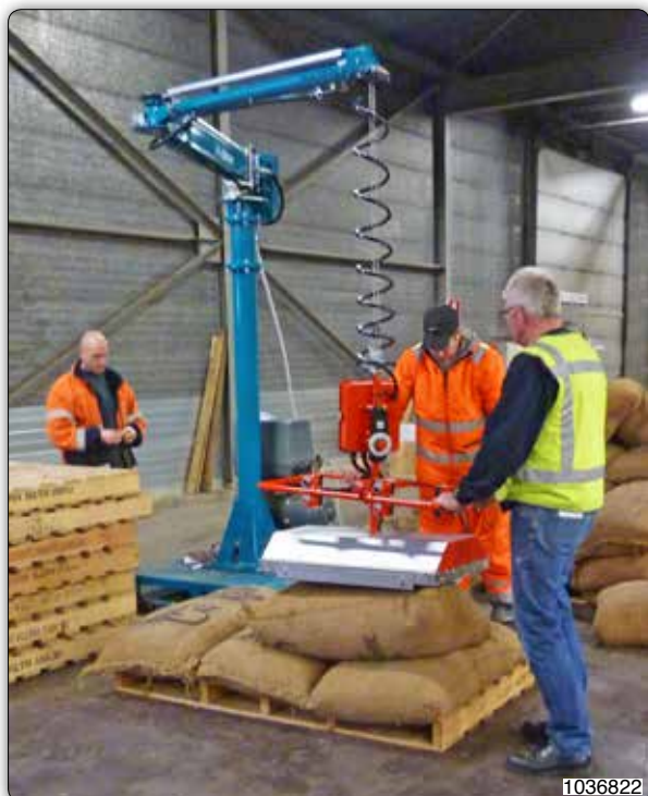
Manipulator with pneumatically actuated grippers, for handling jessian sacks containing coffee, cocoa and similar products.
