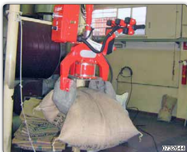
Manipulator with pneumatic clamping grippers which allows the bags to be inclined from the horizontal to the vertical and vice versa.
