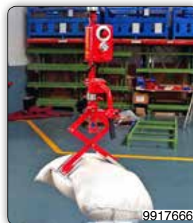
PSC type Partner manipulator, column mounted, equipped with suction head to pick bags from a pallet and to load them to a mixer.
