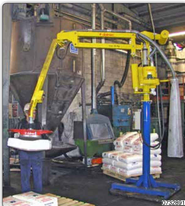
Partner manipulator, column mounted, equipped with suction head to pick bags from a pallet and loading them to a mixer.
