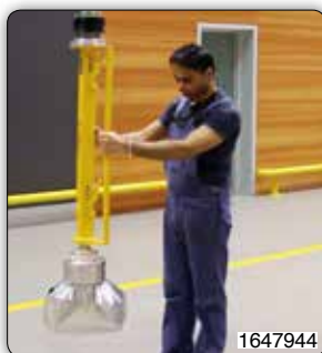
PSC type Partner manipulator, column mounted for palletization/depalletization of bags which are stacked up to about two metres from floor level, fitted with lowered controls.
