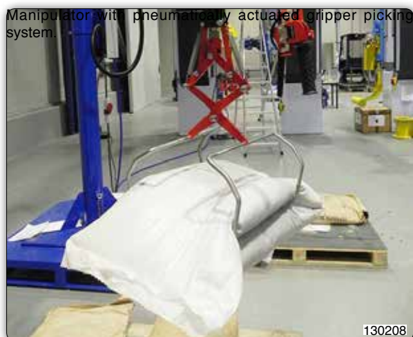
Manipulator with pneumatically actuated grippers, for handling jessian sacks containing coffee, cocoa and similar products.
