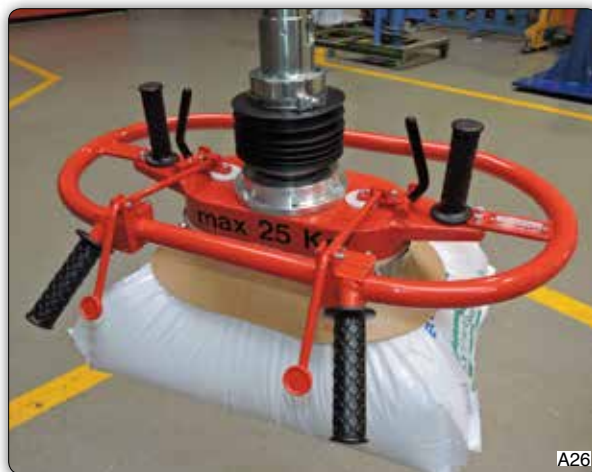
Suction cup for bags complete with rubber lip and lowered controls.
