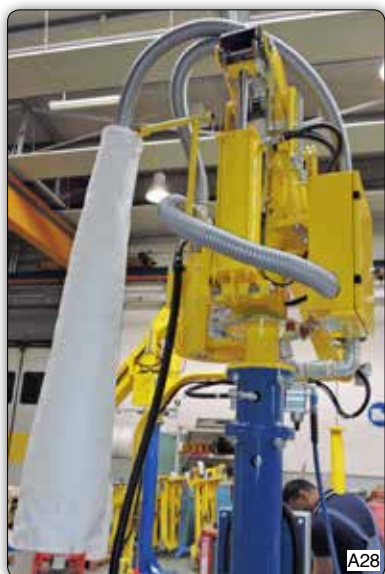
Dust recovery filter mounted on the exhaust piping of the vacuum generator.
