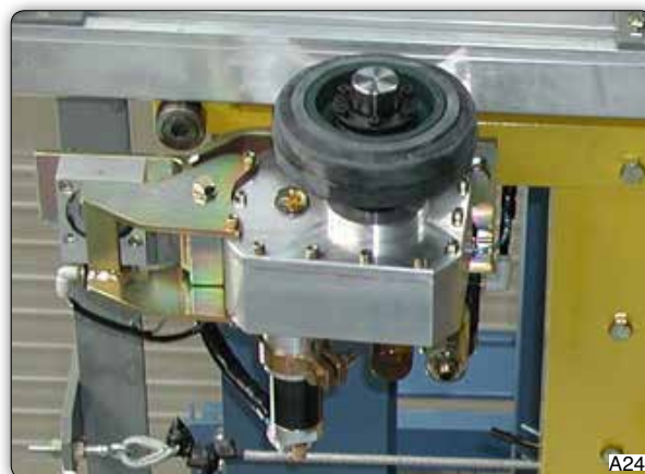
Pneumatic motorization of the translation trolley, composed of a pneumatic motor reducer unit with dragging rubber wheel, complete of filter/lubricator, pressure regulator and push buttons controls for the back and forth running.
