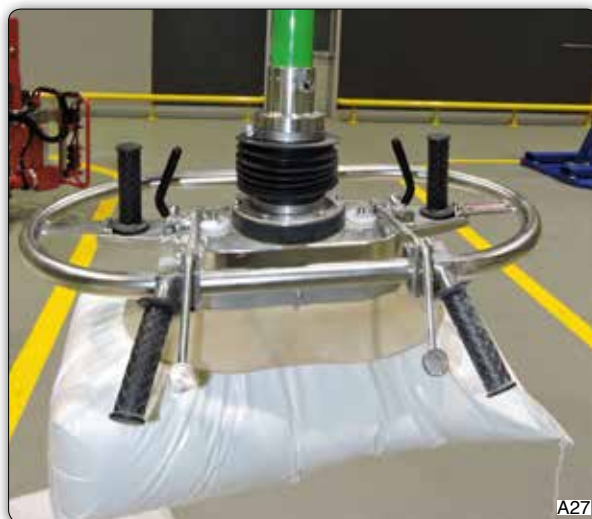
Suction cup stainless steel for bags complete with rubber lip and lowered controls.
