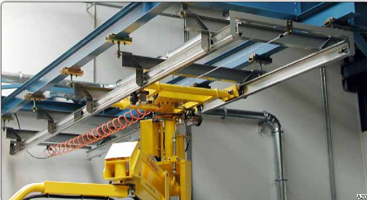
Overhead tracking system complete of end buffers and composed of two special U shaped profiles in special aluminium alloy, with steel runways and connection and stiffening ribs every 2 mt.
