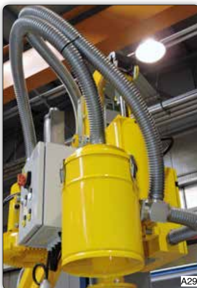
Drum filter, attached to the suction piping of the vacuum generator, used to retain the sucked dust.
