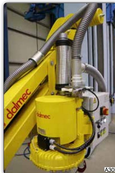
Silencer mounted on the exhaust pipe of the vacuum generator, used to reduce the noise level by 3 dB(A), from 74 to about 71.
