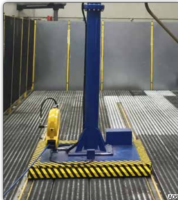
Motorized trolley running on floor built-in runway.
