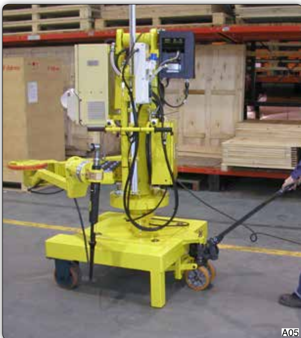
Portable baseplate with trolley for manual displacement.
