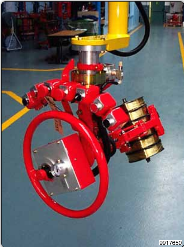
Manipulator with pneumatic jaws for picking multiple coils, with manual rotation of 90°.
