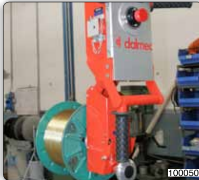
PMC type Partner manipulator, column mounted, equipped with pneumatic action tooling for picking coils of wire on the central belt, with the option of pneumatic inclination from the horizontal to the vertical.
