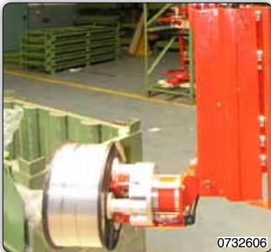
PMC type Partner manipulator, column mounted, equipped with pneumatic action tooling for picking coils of wire on the central belt, with the option of pneumatic inclination from the horizontal to the vertical.
