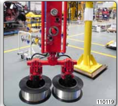
PMC type Partner manipulator, column mounted, equipped with pneumatic action tooling for picking coils of wire on the central belt, with the option of pneumatic inclination from the horizontal to the vertical.
