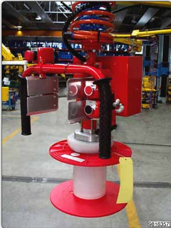
Manipulator with expanding mandrel for picking coils via the core.
