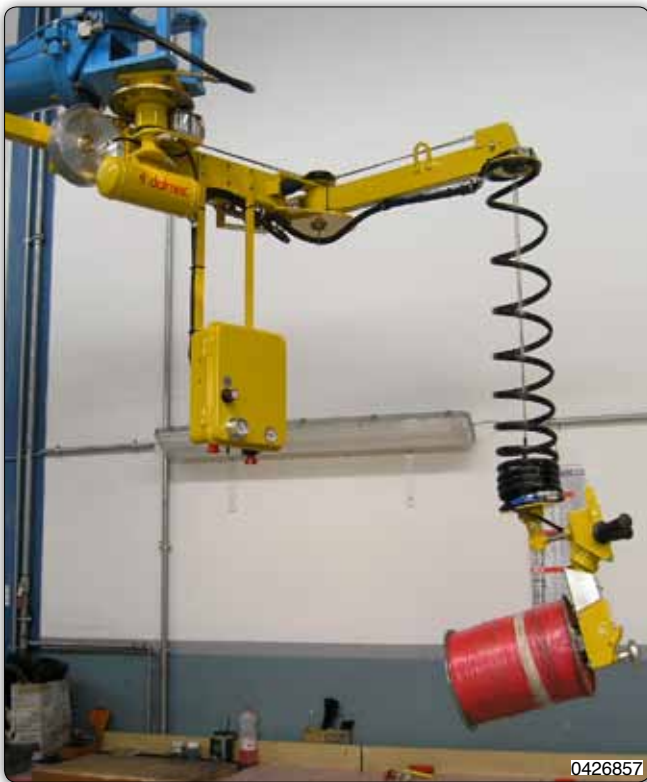
SPF type Speedyfil manipulator, fixed overhead tooling model, fitted with special tooling for picking via an expanding mandrel gripping in the core and manual inclination at 90°. The tooling design caters for automatic picking and release of the coil.
