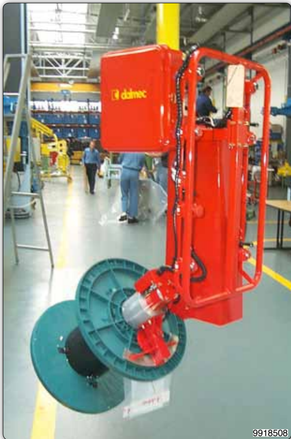
Manipulator with expanding mandrel for gripping in the reel's core, with pneumatic 90° inclination.
