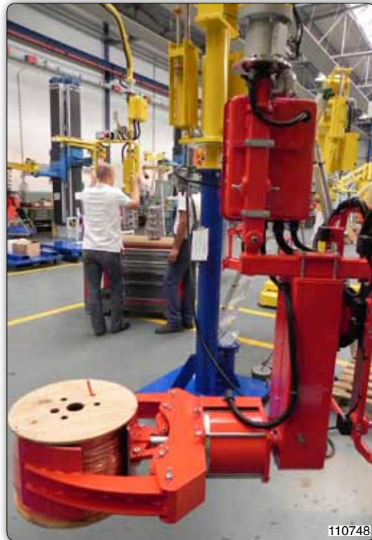
PMC type Partner manipulator, column mounted, provided with gripper tooling to pick metal coils on their central belt.
