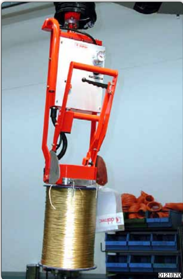
Manipulator designed to pick on the coil's flange with pneumatically actuated tooth, with manual inclination of the coil from the vertical axis to 60°.
