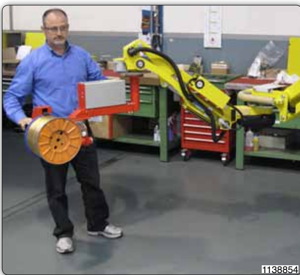
Manipulator especially designed with tooling for picking coils on flange with fixed sector and pneumatically actioned tooth, with manual inclination of the coil.
