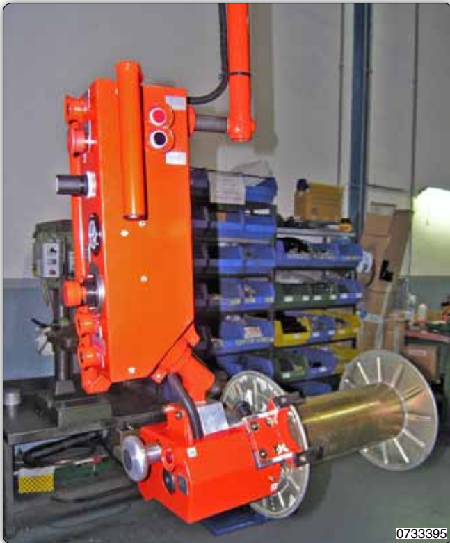
Pneumatic system for picking and moving metal coils. Picking is effected on the flange and the inclination of the coil from the horizontal to the vertical axis is manual.
