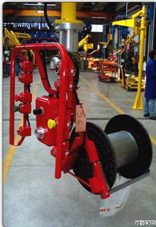
Manipulator fitted with fork-type for handling coils via the flange. Part-present sensors are fitted to the head.
