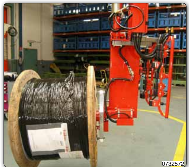
PMC type Partner manipulator, column mounted, fitted with expanding mandrel for gripping bobbins.
