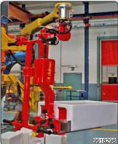
Manipulator with forks type tooling for handling sinks.
