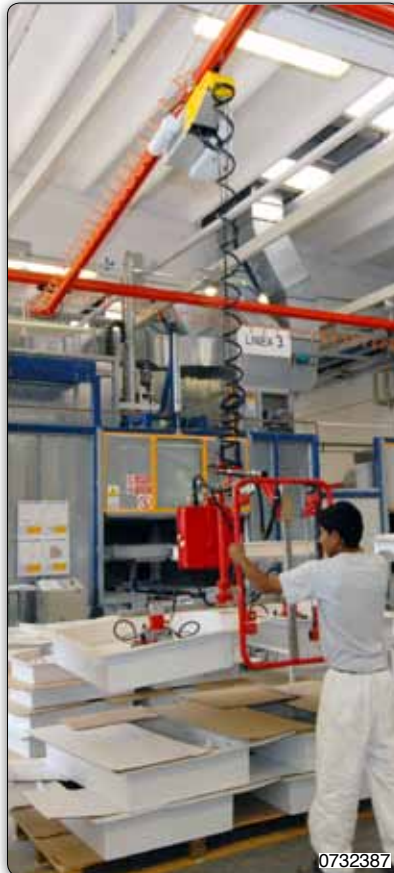
Minipartner manipulator, overhead trolley mounted with suction cups tooling for handling of fiberglass shower trays.
