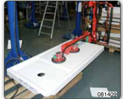
Manipulator with suction cups tooling (Venturi) for gripping shower plates.
