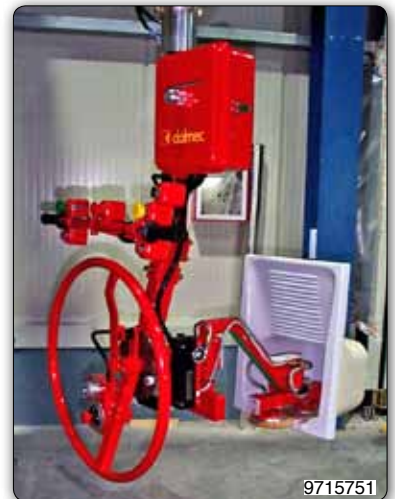
Manipulator with suction cups tooling (Venturi) for gripping and manual rotation of sinks.
