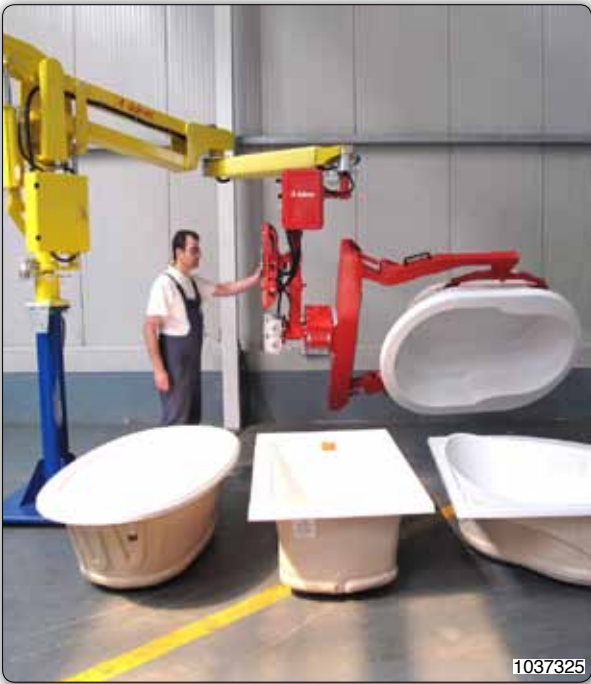
Manipulator with jaws tooling for gripping and rotation of bathtubs.
