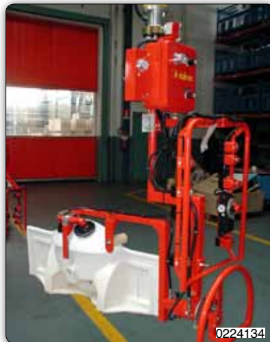
Manipulator with suction cups tooling (Venturi) for gripping and manual rotation of sinks.
