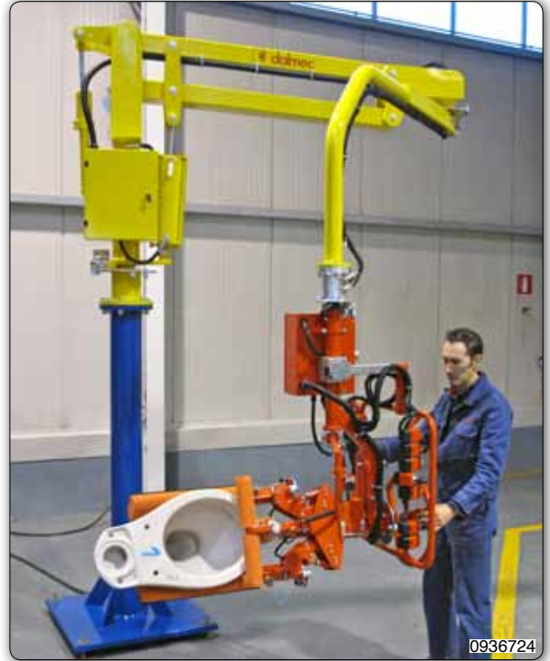
Manipulator with pinch jaws covered with sponge rubber for gripping and manual rotation of WC.
