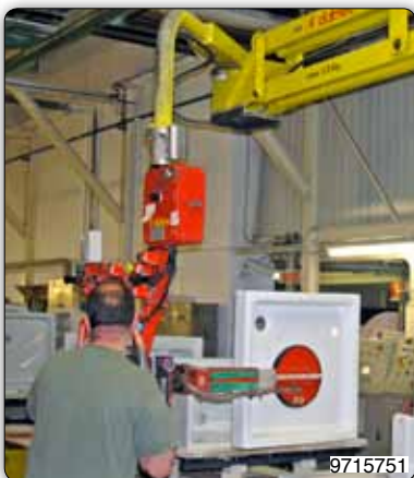
Manipulator with suction cups tooling (Venturi) for gripping shower trays.
