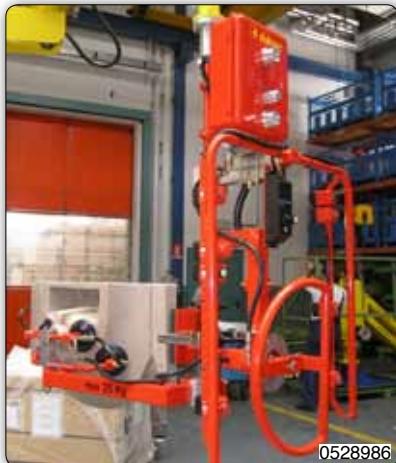
Manipulator with adjustable suction cups tooling (Venturi) for gripping and manual rotation of raw sinks.
