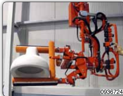
Pinch jaws tooling covered with sponge rubber for handling and manual rotation of WC.
