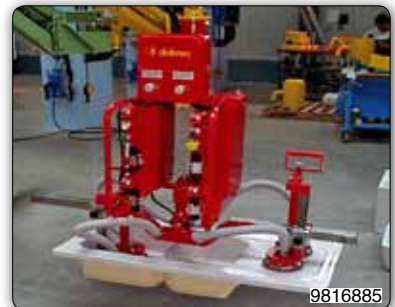
Manipulator with adjustable suction cups tooling (Venturi) for handling and inclination of sinks.
