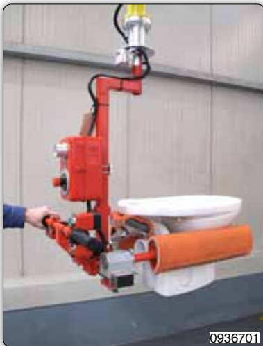
Tooling with adjustable forks covered with sponge rubber for the handling of wc.
