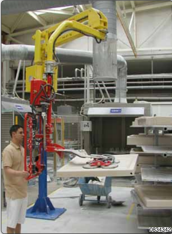
PMC Partner manipulator, column mounted, equipped with suction cups tooling (Venturi) for gripping and manual rotation of raw shower plates.
