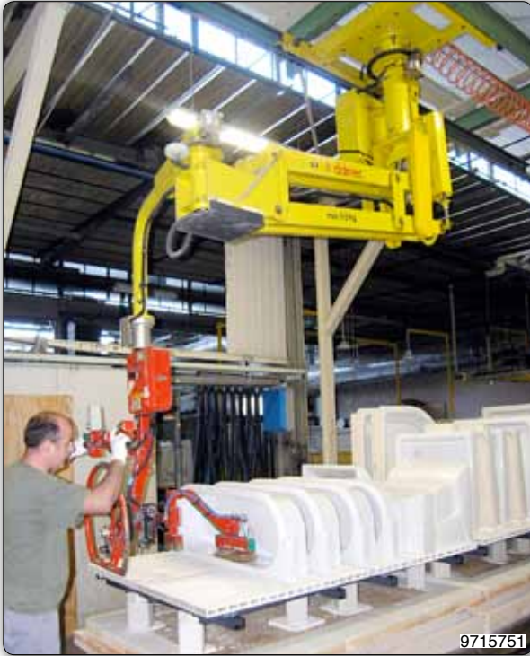
PMS Partner Manipulator, overhead trolley mounted, with interchangeable suction cups tooling for gripping and handling sinks having different dimensions.
