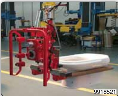
Adjustable forks tooling for handling WC.
