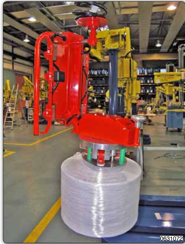
PMC type Partner manipulator, column mounted, equipped with an expanding mandrel for handling and 90° inclination of reels. The manipulator has a load cell for checking the weight of the reels.
