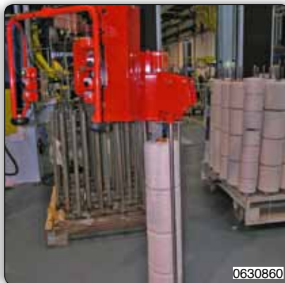
Pneumatic expansion mandrels or pinch jaws toolings for gripping, handling and inclination of reels having different dimensions and characteristics.
