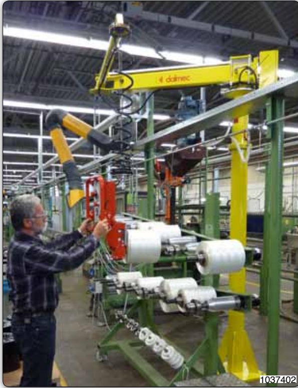
PFC type Posifil manipulator, column mounted unit, with expanding tooling for picking bobbins from a pallet and placing them horizontally to an unwinding machine.
