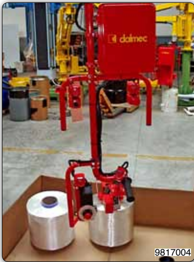
Pneumatic expansion mandrels or pinch jaws toolings for gripping, handling and inclination of reels having different dimensions and characteristics.
