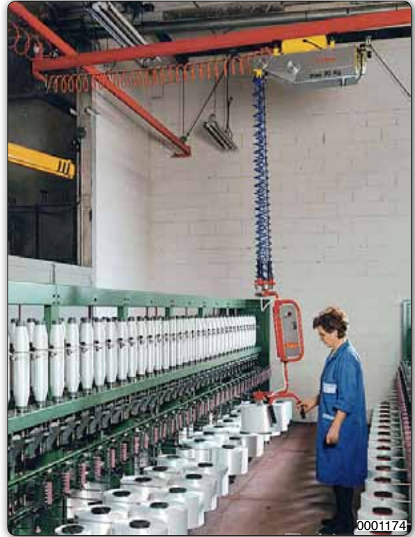
MPS Minipartner manipulator, overhead trolley mounted running in a bridge crane, fitted with pneumatic tooling head for the handling of reels.
