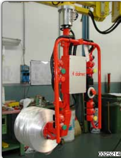
Pneumatic expansion mandrels or pinch jaws toolings for gripping, handling and inclination of reels having different dimensions and characteristics.
