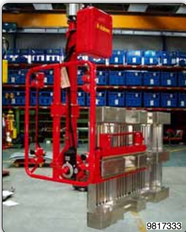
Manipulator with particular forks for gripping and handling stainless steel pallets.
