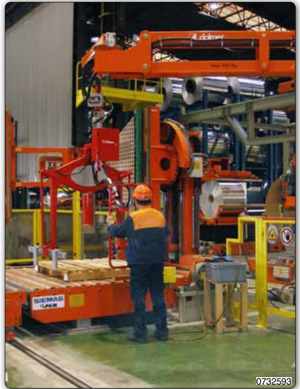
PMC type Partner Manipulator, column mounted with jaws tooling for gripping pallets.
