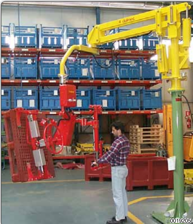
PMC type Partner Manipulator, column mounted with jaws tooling for gripping, pneumatic inclination and manual rotation of plastic pallets.
