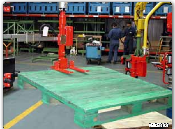
Forks tooling for handling pallets.
