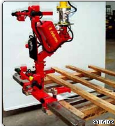
Adjustable forks tooling with block device.
