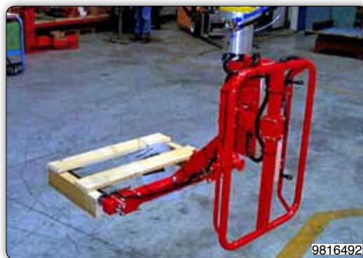
Manipulator with forks type tooling and part presence sensor for handling pallets.
