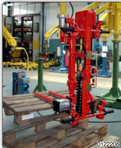
Adjustable forks tooling with pneumatic rotation of the load and telescopic controls.
