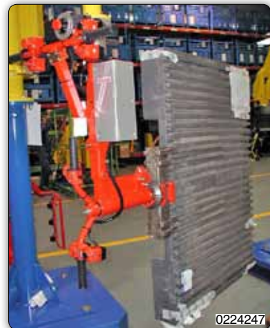
Forks gripping system for particular pallets.
