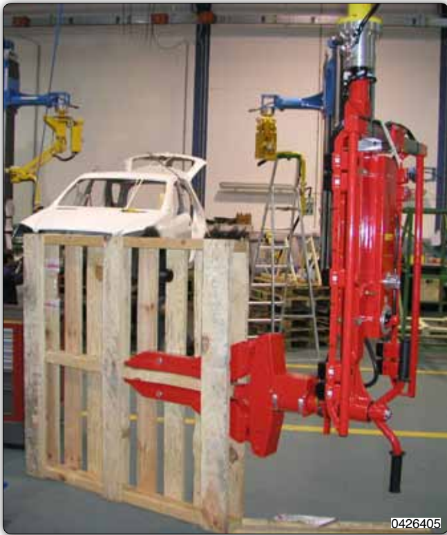
Manipulator with pneumatic tooling with manual of the pallet.
