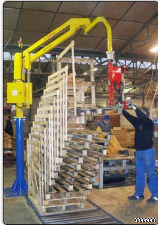
Manipulator with forks tooling for handling pallets.
