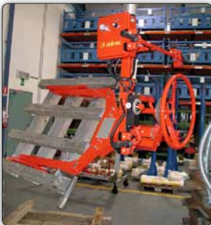
Manipulator with jaws type tooling with manual rotation of the pallet.
