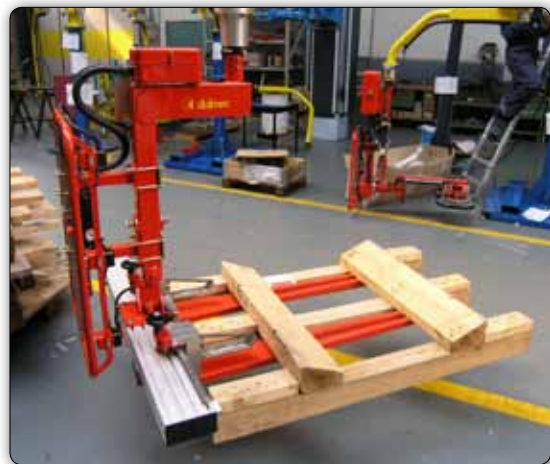
Adjustable forks gripping system for particular pallets.
