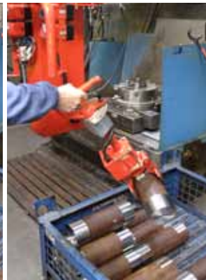
Pinch jaws tooling for the gripping and pneumatic rotation of discs having different forms and weights.
