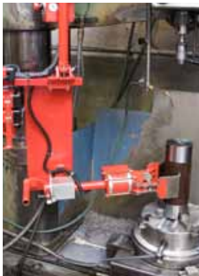
MIS Micropartner manipulator, overhead trolley mounted, with pneumatic tooling for the picking and manual inclination of hubs for use on a machining centre.
