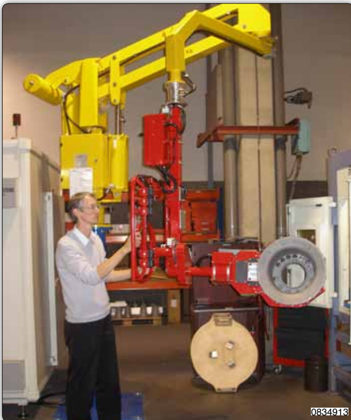
PMC type Partner manipulator, column mounted, with pneumatic tooling for picking mechanical components and manually rotating them through 180°, for use on a machining centre.
