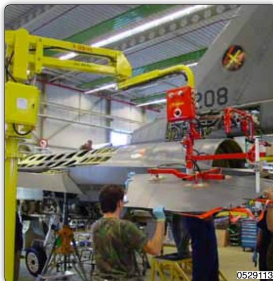
Manipulator with vacuum suction system for moving parts of aircraft wings.
