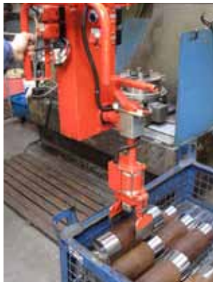
Pinch jaws tooling for the gripping and pneumatic rotation of discs having different forms and weights.
