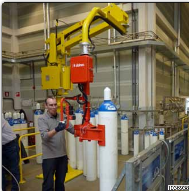
Manipulator with pneumatic gripping tool for picking and 90° pneumatic inclination of cylinders.
