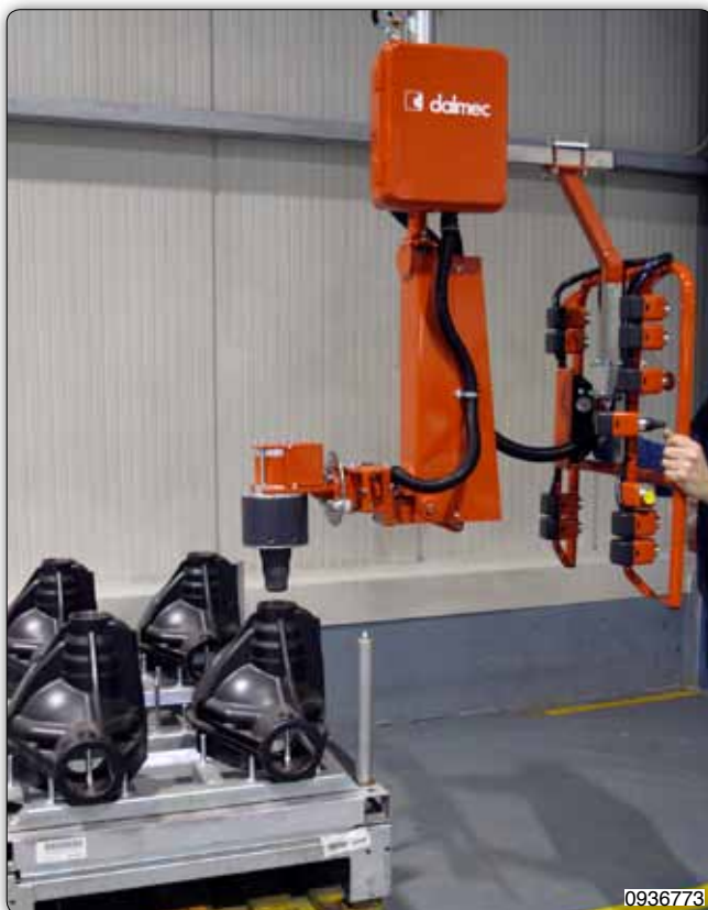
PMC type Partner manipulator, column mounted provided with pneumatic pincer to handle with servo-assisted inclination, gearbox casings to be transported to the die-stamping machine.
