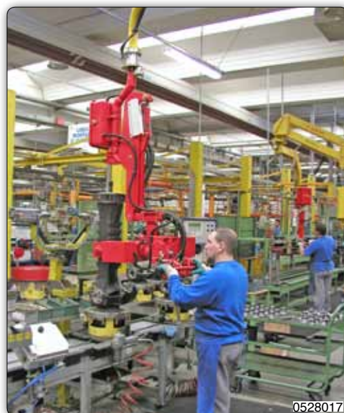
PMC type Partner manipulator, column mounted, equipped with pneumatic tooling to pick, handle and, after a 180° rotation, to place axes on a workbench.
