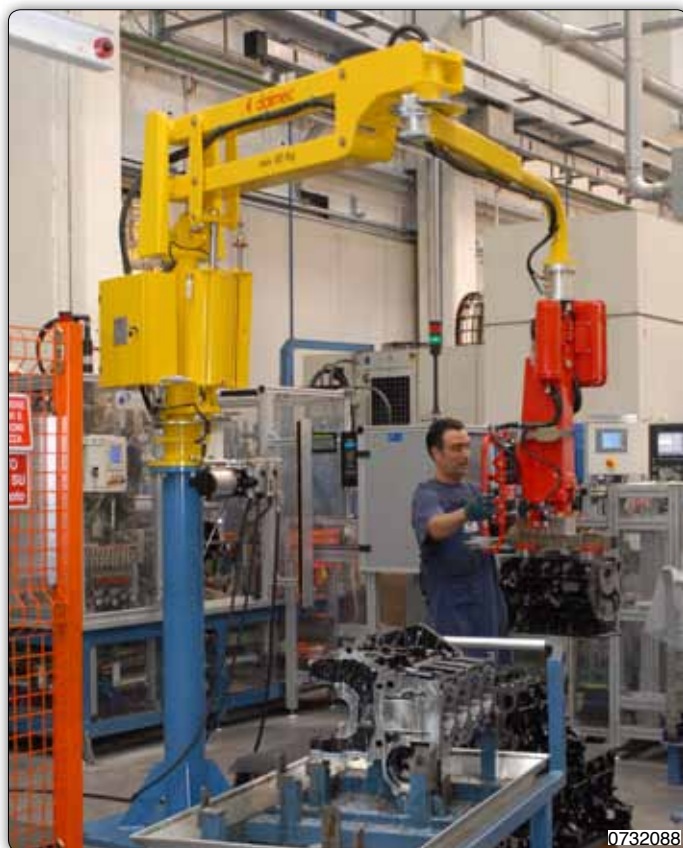
PMC type Partner manipulator, column mounted, used to handle crankcases.
