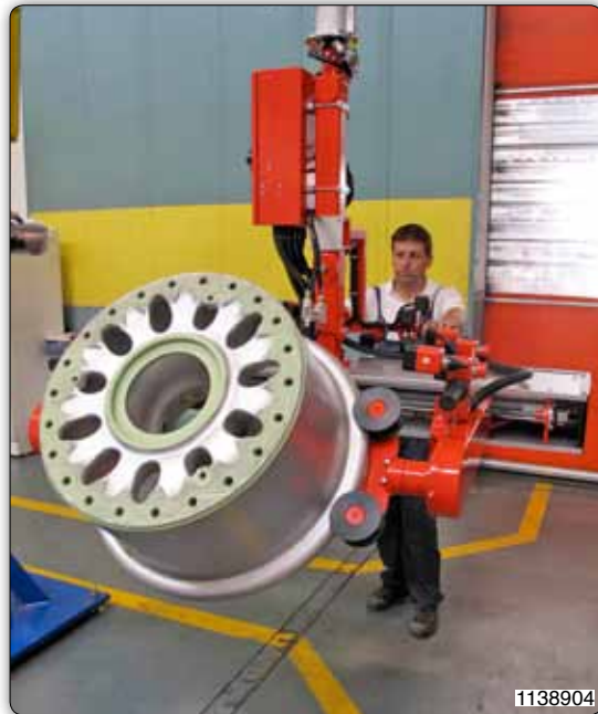
Pinch jaws tooling for the gripping and pneumatic rotation of discs having different forms and weights.
