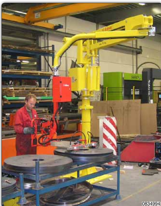
PMC type Partner manipulator, column mounted version, with adjustable suction cups tooling for picking sheets.
