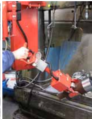
MIS Micropartner manipulator, overhead trolley mounted, with pneumatic tooling for the picking and manual inclination of hubs for use on a machining centre.
