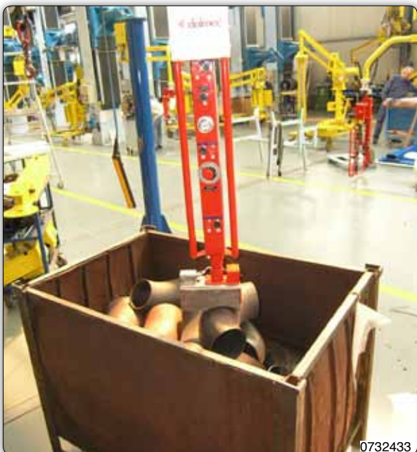
Manipulator with multipolar permanent magnet pneumatically operated, for gripping and lifting steel curves placed jumbled in a container.
