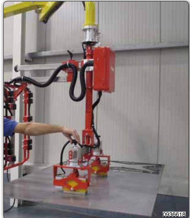
Manipulator equipped with electropermanent magnet for placing steel products on a machine tool.
