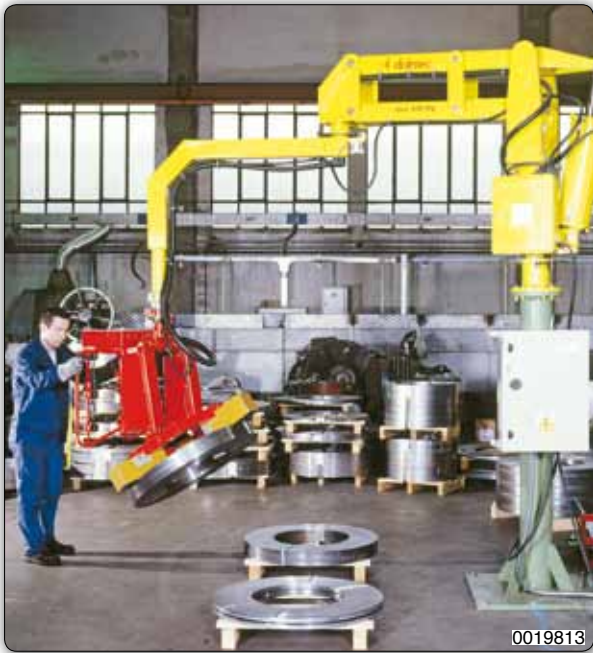
Manipulator with multipolar permanent magnets pneumatically operated for gripping and lifting steel strap rolls. The distance between centres of the magnets is manually adjustable.
