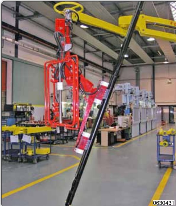
Manipulator with multipolar permanent magnets pneumatically operated designed for picking steel shafts and their inclination through 90°.
