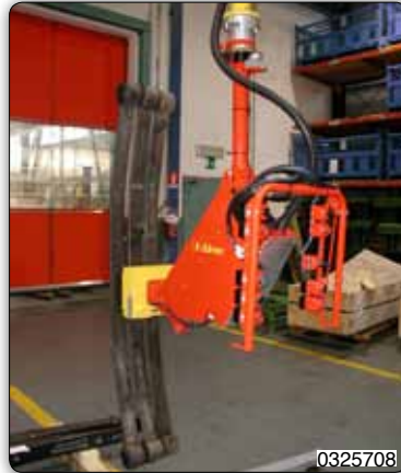
Manipulator equipped with multipolar magnets pneumatically operated for gripping and lifting steel sheets. The distance between centres of the magnets is manually adjustable.
