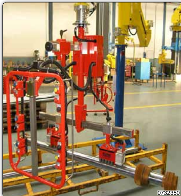
Manipulator equipped with multipolar permanent magnets pneumatically operated, for gripping and lifting steel shafts.
