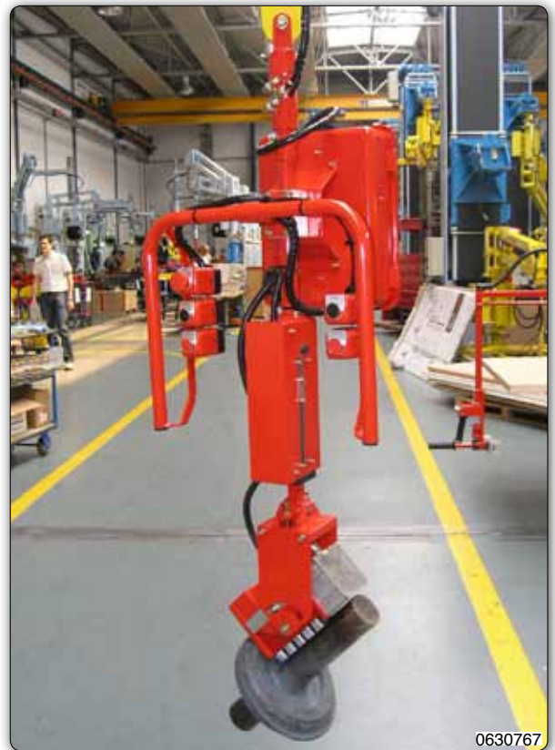
Manipulator with multipolar permanent magnet pneumatically operated, for gripping and lifting mechanical parts placed jumbled in a container.
