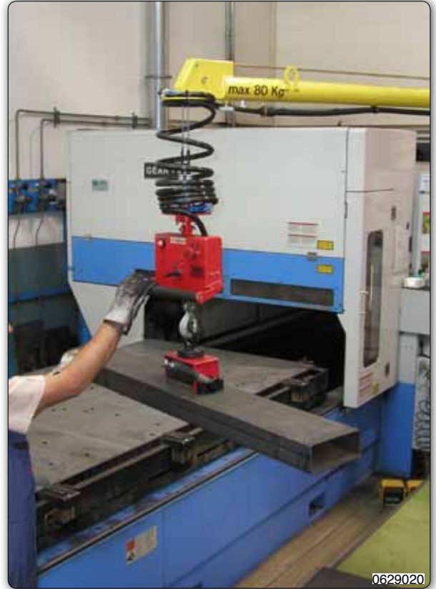
Manipulator with bipolar permanent magnet manually actuated, equipped with anti-release safety device which prevents the tooling from releasing the load before it is correctly in place.
