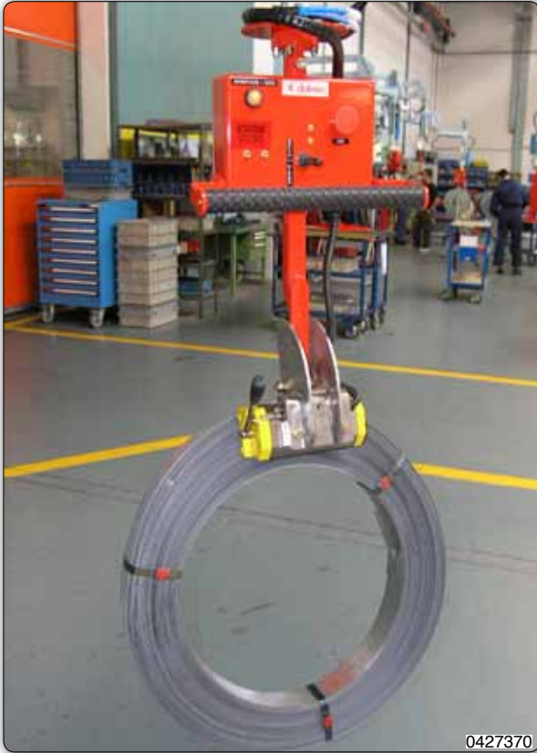
Manipulator equipped with bipolar permanent magnet manually operated, designed to grip metal strap rolls positioned horizontally and then incline them manually through 90°.
