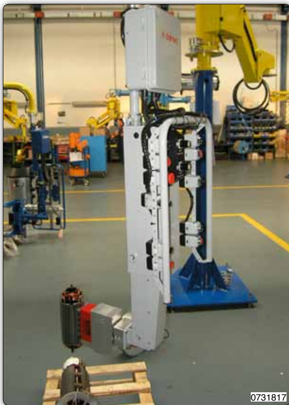
Manipulator equipped with a magnet gripping tool for handling rotors on the outside diameter with pneumatic inclination.
