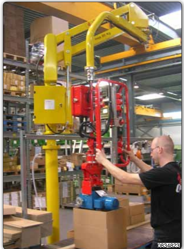
Manipulator equipped with jaws tooling to grip the electric motors on the outside diameter, with the manual rotation of the motor.
