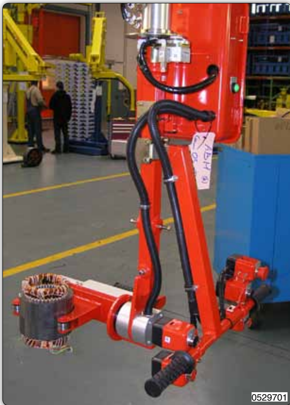
Manipulator equipped with gripping jaws for handling electric stators on the outside diameter, with a manual rotation of the stator.
