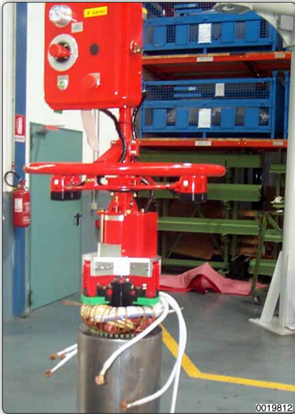
Manipulator equipped with jaws gripping tool for handling stators in the inside diameter.
