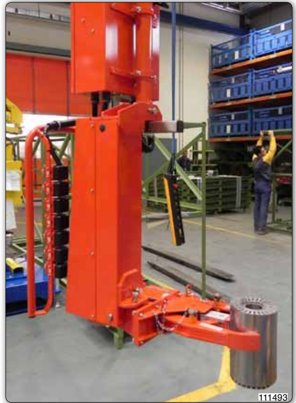
Manipulator equipped with gripping jaws tool for handling rotors on the outside diameter with pneumatic inclination.
