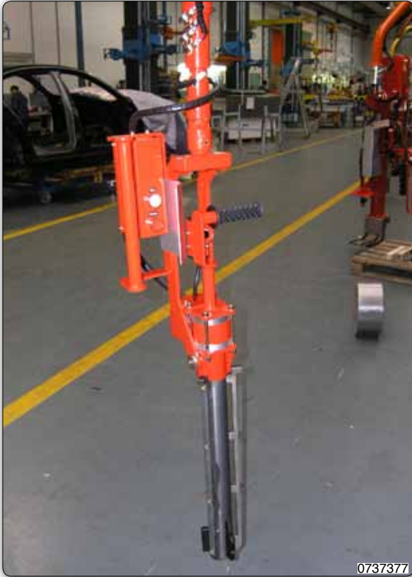
Manipulator equipped with expanding mandrel tooling for gripping packs of laminations, with manual inclination up to ~60°.
