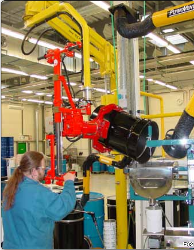
PMC type Partner manipulator, column mounted, designed for picking and emptying drums.
