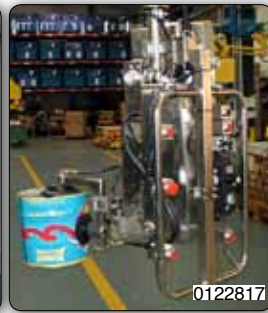
Pneumatic tooling head for handling three drums at the same time.
