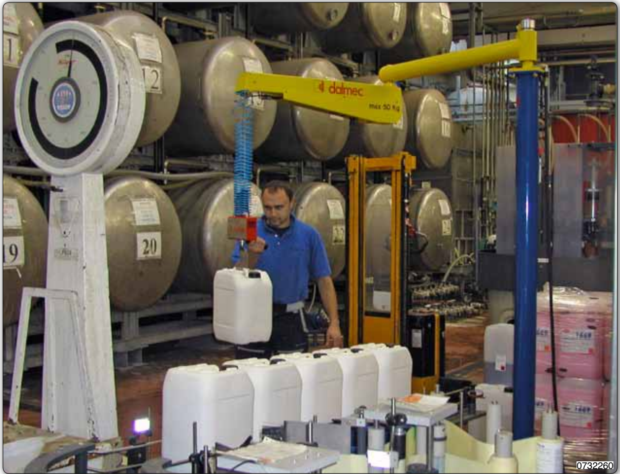
PVC type Posivel manipulator, column design, equipped with specially shaped hook designed for palletizing jerrycans.
