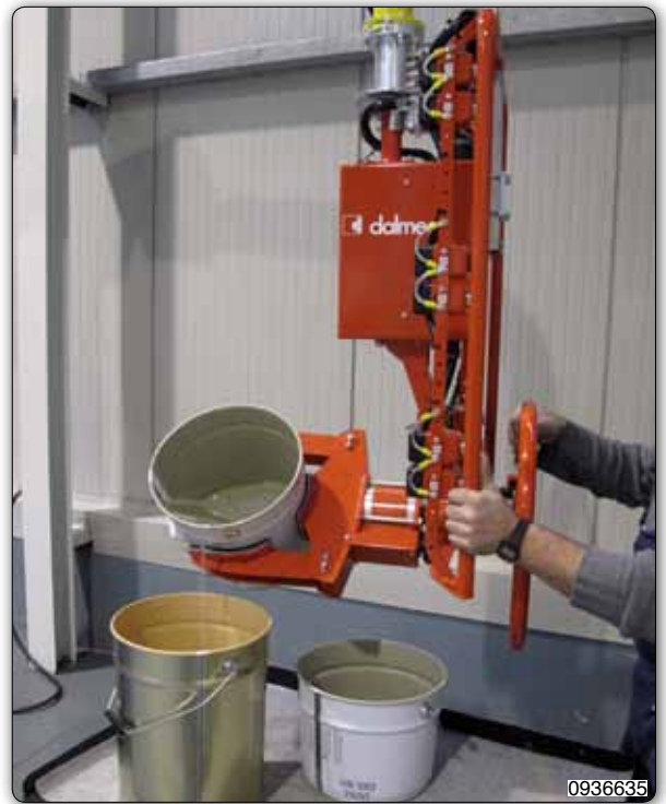
PMC type Partner manipulator, column mounted version, designed for picking and emptying drums.
