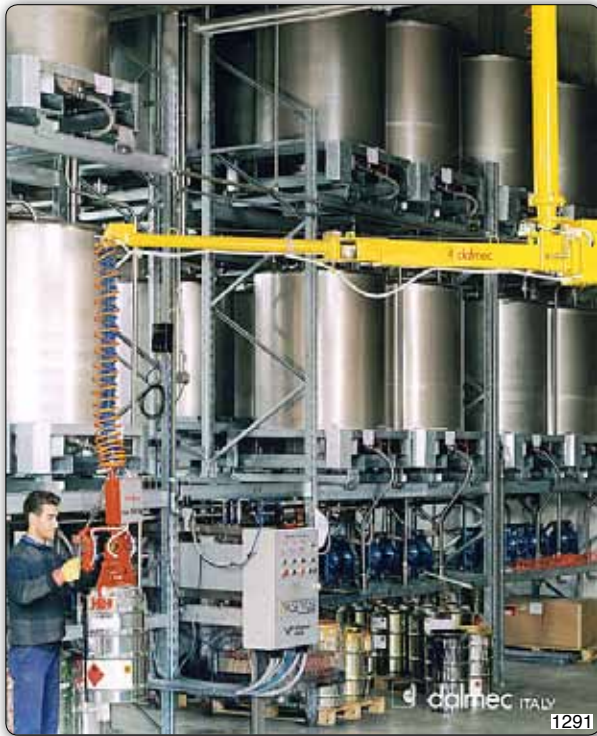
PFF type Posifil manipulator, fixed overhead version for handling metal drums.
