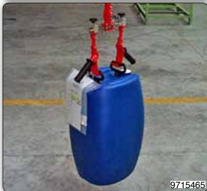
Manipulator equipped with moulded hooks for gripping and handling pails.
