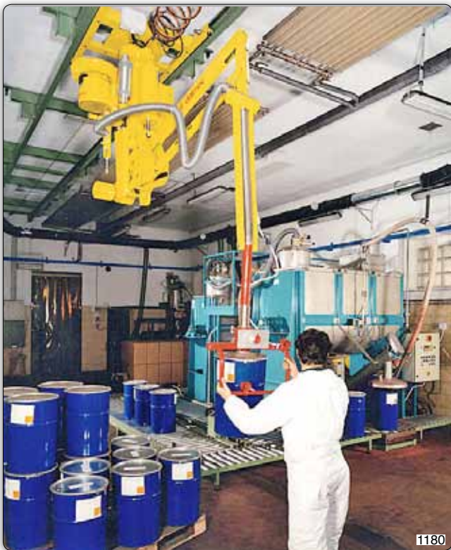
PSS type Partner manipulator, overhead trolley mounted version, with a vacuum tooling head, vacuum being generated by "Venturi" ejector.
