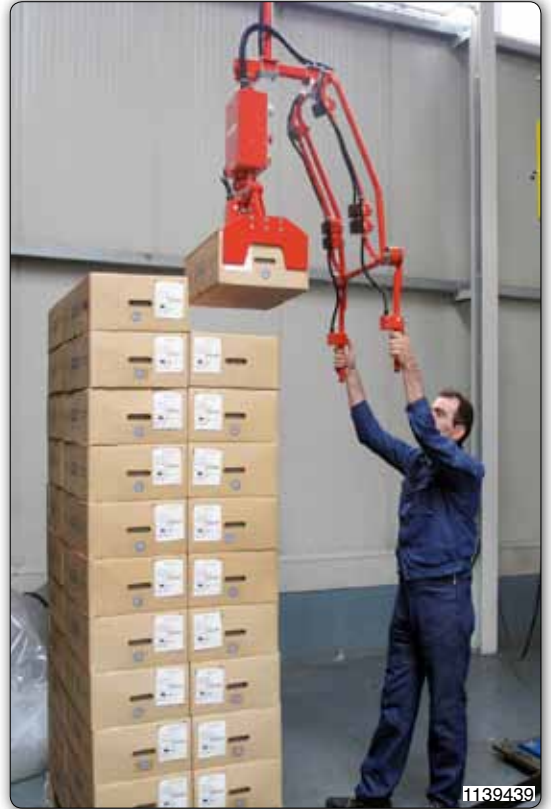
Manipulator equipped with special pneumatic gripping tooling whose particular structure allows the operator to pick boxes from a high stack on a pallet.
