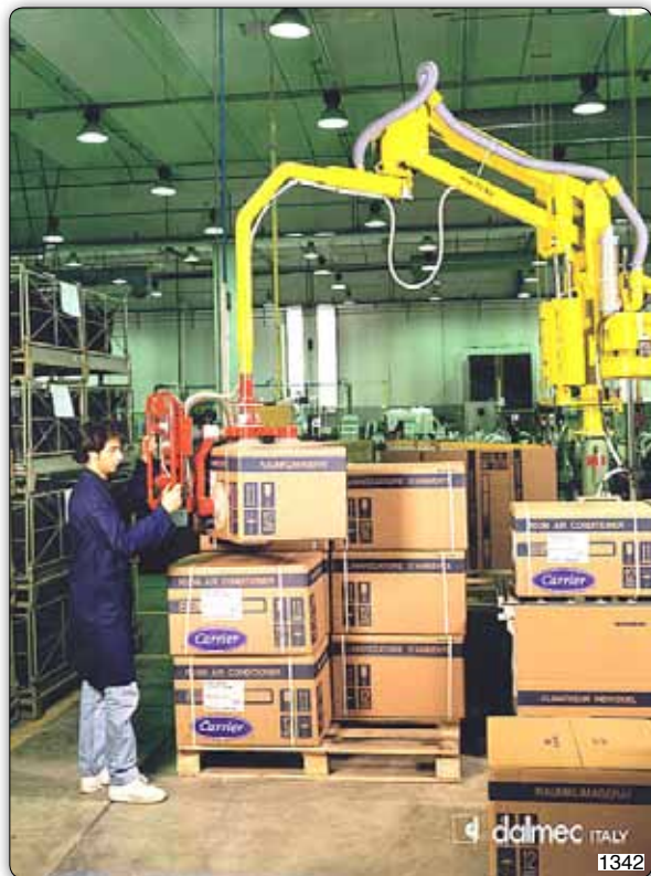
PMC type Partner manipulator, column mounted, with suction gripping system, a popular design, commonly used for moving packing boxes from a conveyor belt to a pallet.
