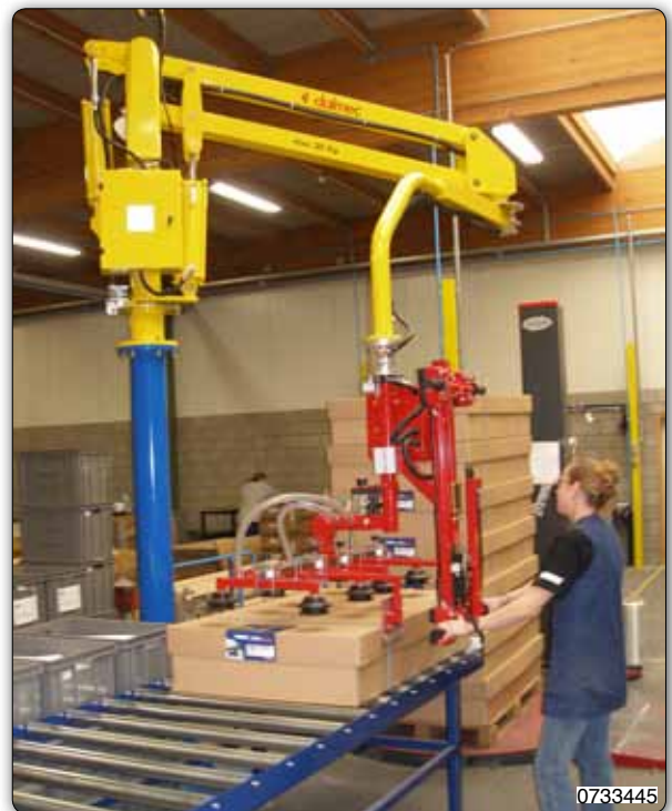
PMC type Partner manipulator, column mounted, equipped with suction system to grip and handle cardboard boxes from the packaging lines to pallets.
