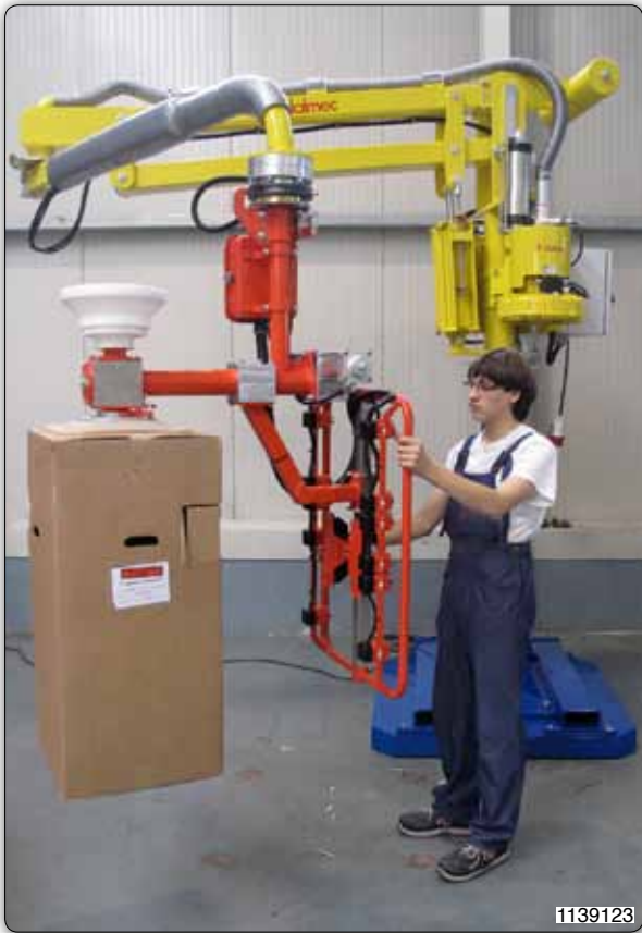
PMC type Partner manipulator, column mounted on portable baseplate, equipped with double suction cups gripping system for gripping industrial lamps and their packaging.
