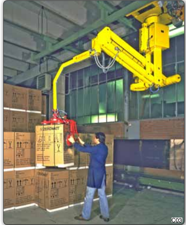
PMS type Partner manipulator, overhead trolley mounted, suitable for stacking boxes containing a variety of washing machines which arrive from the packaging line. A pneumatic motor drive is also fitted to the system, which runs in Dalmec overhead tracking.
