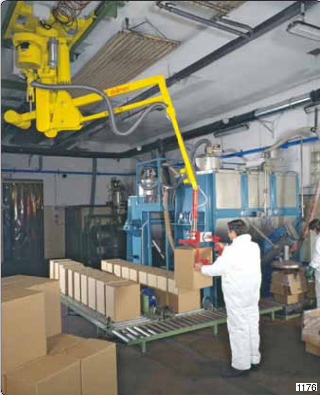
PSS type Partner manipulator, overhead trolley mounted version, fitted with vacuum tooling for gripping boxes from one packaging line and positioning the same on a pallet. The overhead tracking system is manufactured by Dalmecc.
