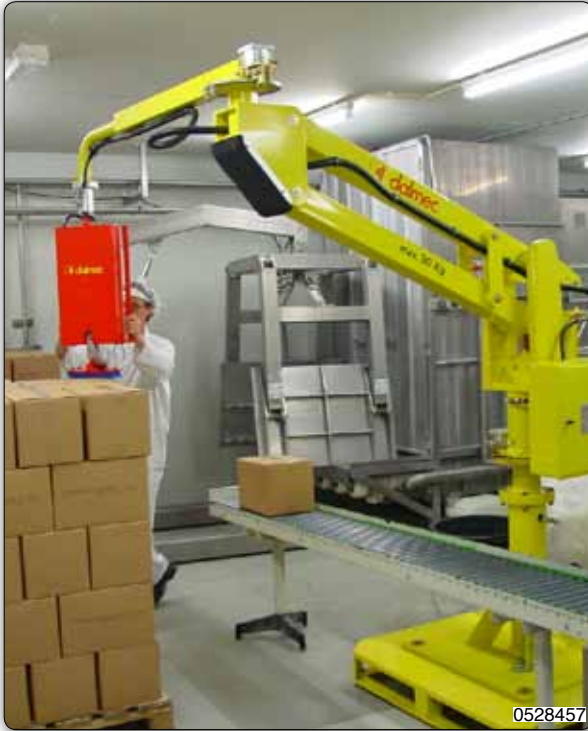
PMC type Partner manipulator, low profile model, fitted with suction head for gripping cardboard boxes and designed to operate in an area with a low ceiling.
