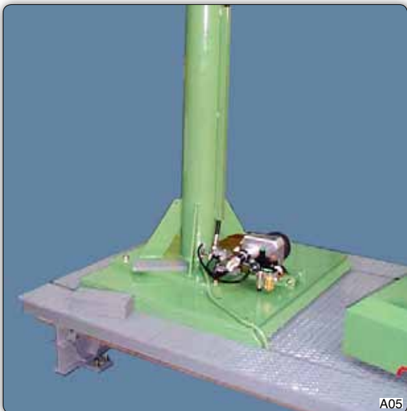
Floor built-in runway with pneumatic motor.
