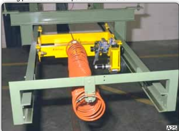
Compressed-air station to feed the Manipulator along the whole existing tracking system, composed of an air spiral, supporting cable and drive pulley.
