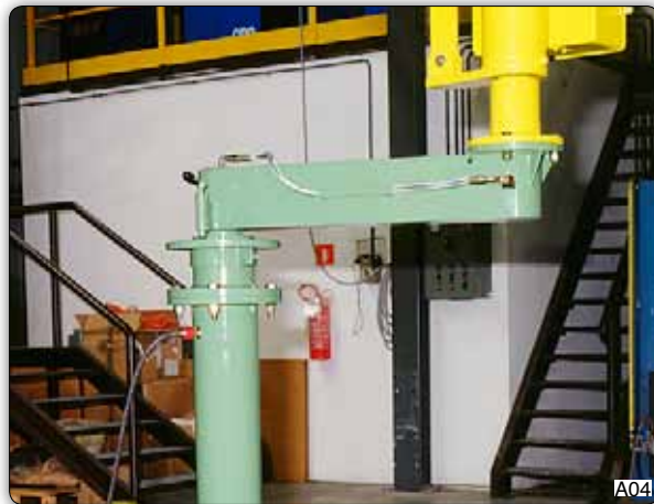
Off-set column to increase the working area of the Manipulator, complete with mechanical stop every 45°.
