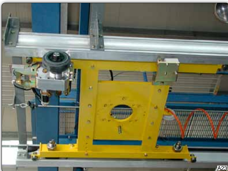
Trolley complete of wheels for the manual running in the tracking system and of drilling plate for the Manipulator attachment.
