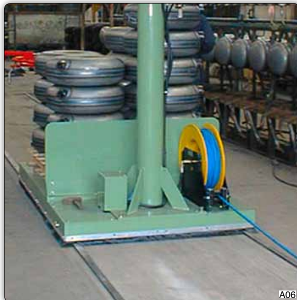
Lengthened motorized trolley running on rails to transport the products to be handled.
