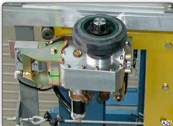
Pneumatic motorization of the translation trolley, composed of a pneumatic motor reducer unit with dragging rubber wheel, complete of filter/lubrificator, pressure regulator and push buttons controls for the back and forth running.
