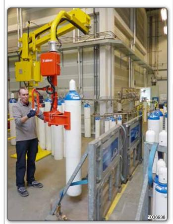
Manipulator with pneumatic tooling for gripping and inclination of cylinders having different dimensions.
