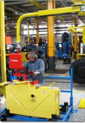
Manipulator with pneumatic tooling for gripping and handling of tanks for industrial vehicles.
