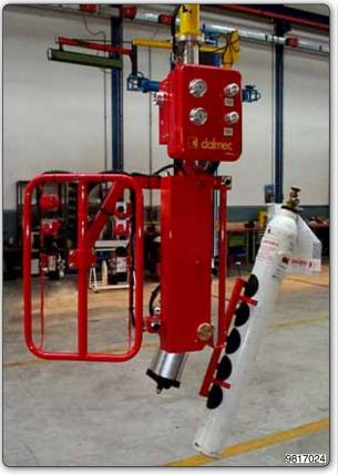
Manipulator with suction cup tooling (Venturi) for gripping and inclination of cylinders.
