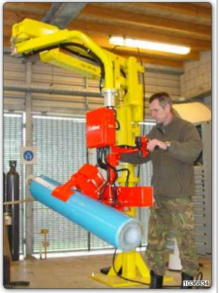
Manipulator with pneumatic tooling for gripping,  $90^{\circ}$  pneumatic inclination and  $180^{\circ}$  manual overturning of cylinders of different dimensions.
