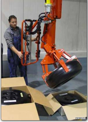
Manipulators equipped with pneumatic tooling for gripping and manual rotation of round tanks.
