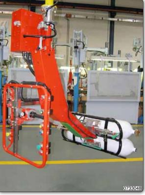
Manipulator with suction cups tooling (Venturi) for gripping and inclination of tanks.
