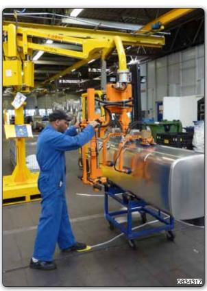
Manipulator with suction cups tooling (Venturi) for gripping and handling of tanks.
