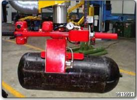
Manipulator with suction cup tooling (Venturi) for gripping and releasing the LPG tanks into the car.
