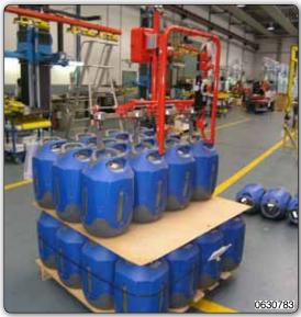
Manipulator with hooks tooling for gripping one or two cylinders.
