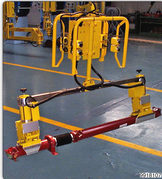
Manipulator with adjustable jaws and double gripping head tooling for handling transmission shafts.
