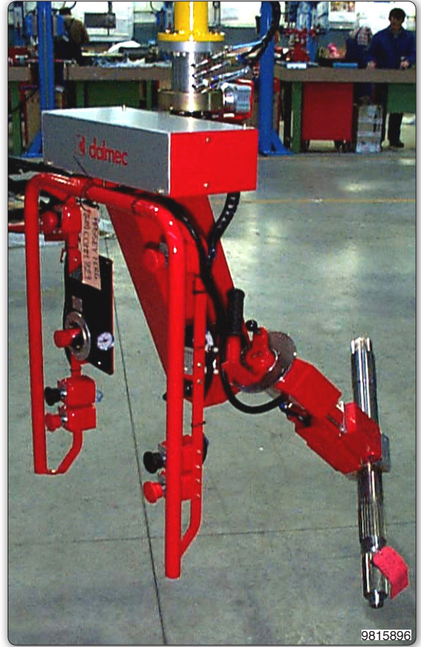
Manipulator with pneumatic tooling for gripping, inclination and rotation of transmission shafts.
