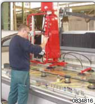
Adjustable suction cups tooling for handling and 90° pneumatic inclination of glass sheets.
