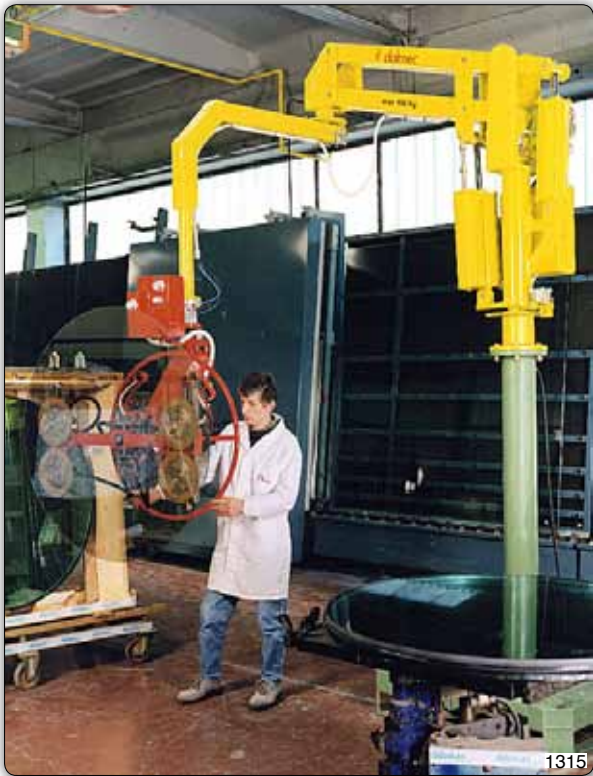
PMC type Partner manipulator, column mounted, equipped with suction system to pick plate glasses from a trolley, and following pneumatically assisted inclination, to place the plate on a table, or vice versa. The tooling also allows the manual rotation through an angle of 360° about the horizontal axis.
