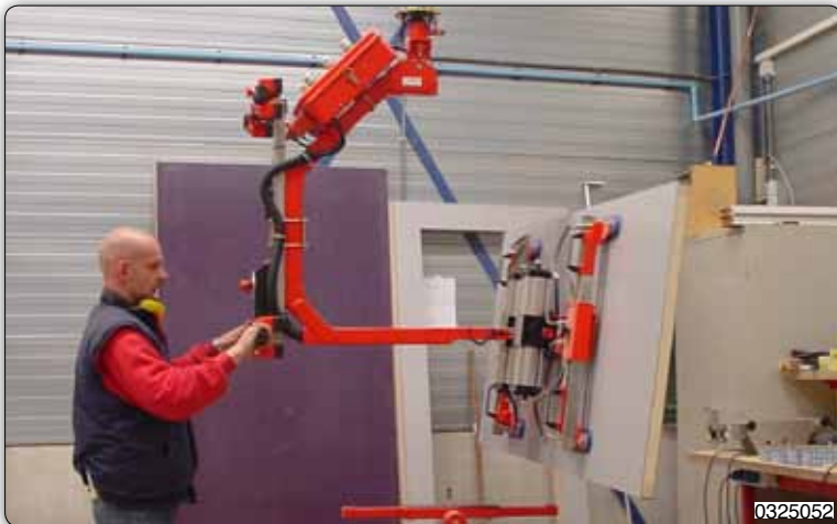
Suction tooling for handling and 180° pneumatic rotation of wooden panels with different dimensions. The position of the suction cups is manually adjustable.
