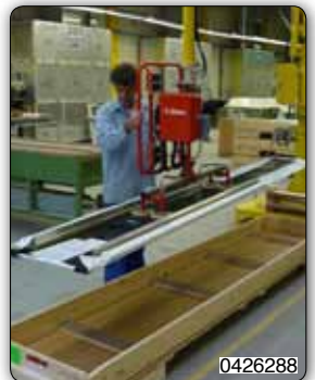
Vacuum suction systems and pneumatic or manual inclination/rotation for handling different types of products.
