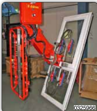
Adjustable suction cups tooling pneumatic inclination for handling door and window frames.
