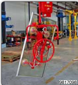
Suction cups tooling for handling and 360° manual rotation of panes of glass.
