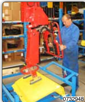
Vacuum suction systems and pneumatic or manual inclination/rotation for handling different types of products.
