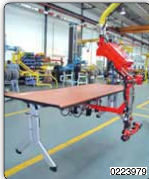
Vacuum suction systems and pneumatic or manual inclination/rotation for handling different types of products.
