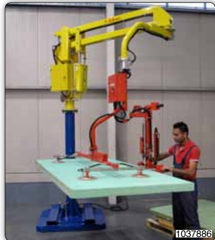
Manipulator with suction tooling for gripping insulating boards.
