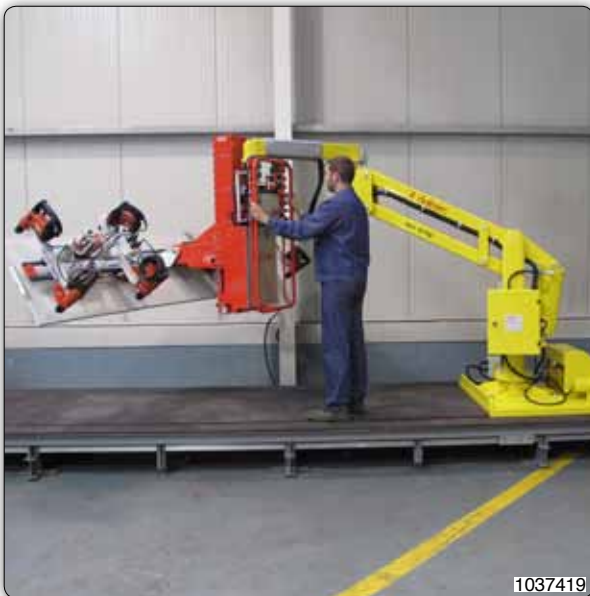
PMC type Partner manipulator, column mounted, equipped with adjustable suction cups tooling for handling special panels.
