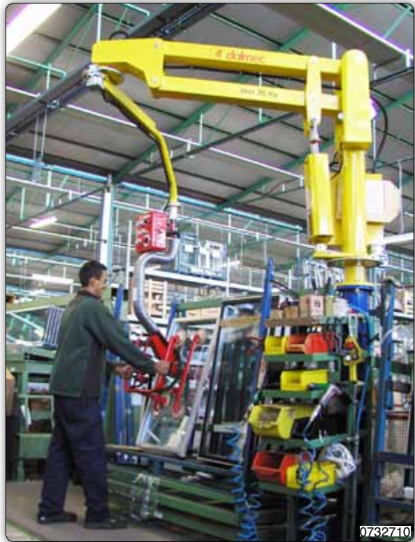
PMC type Partner manipulator, column mounted unit, equipped with a suction system for picking panes of glass from a conveyor and for positioning them on a frame. Vacuum is generated by an electric pump fitted on the side of the manipulator.
