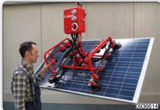
Vacuum suction system with manual inclination for gripping and handling photovoltaic panels.
