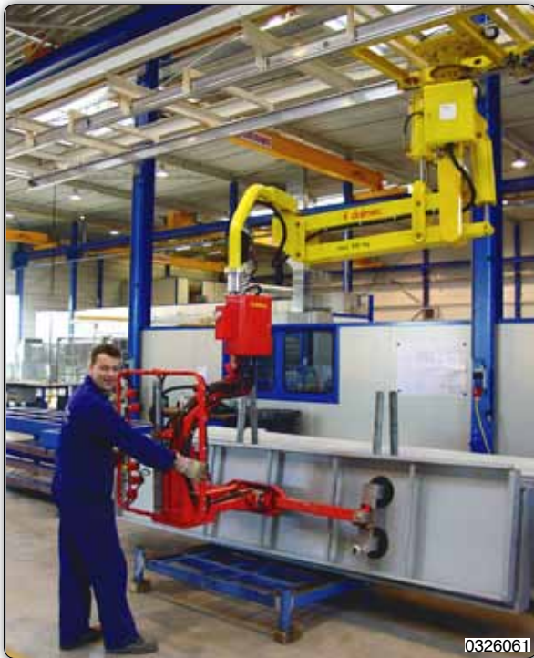
PMS type Partner manipulator, overhead trolley mounted with motorised pneumatic drive, fitted with adjustable suction cups tooling for handling and inclination of big panels.
