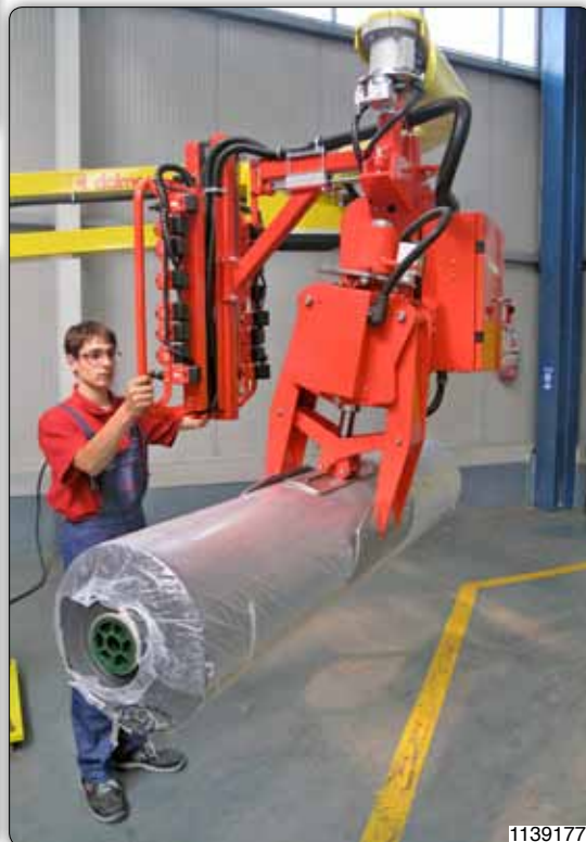
PMC column-type Partner, with pneumatic gripping jaws for handling rolls about their external diameter.
