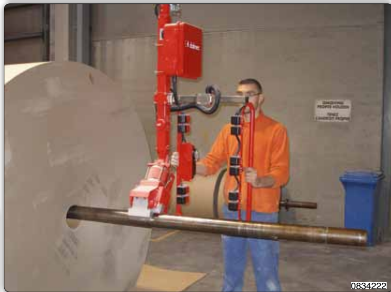
Manipulator complete with pneumatic gripper for picking and handling carrier shafts.
