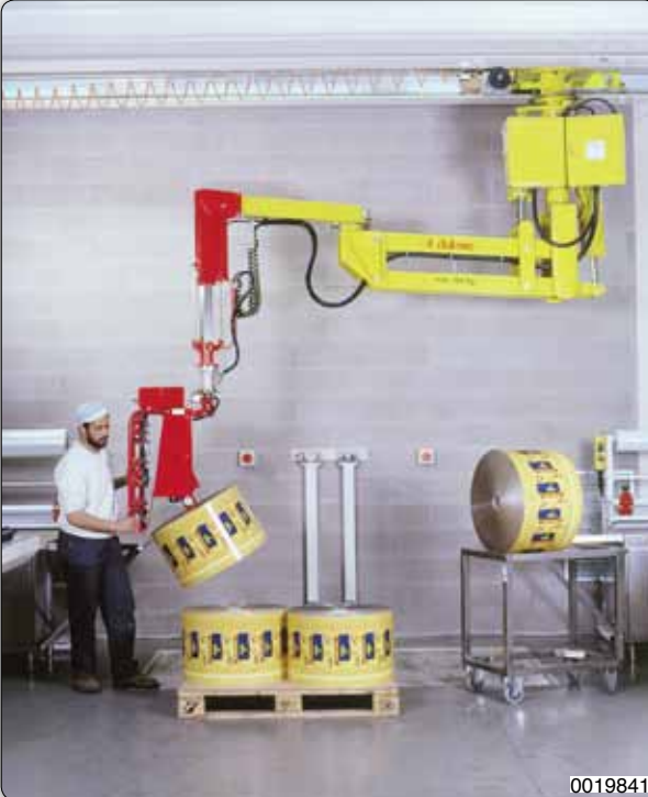
PMS type Partner manipulator, overhead trolley mounted unit, with pneumatic power drive, designed for lifting reels of plastic film from a cradle to a pallet. The tooling head consists of a pneumatically expanding mandrel with 90 degree pneumatic inclination.
