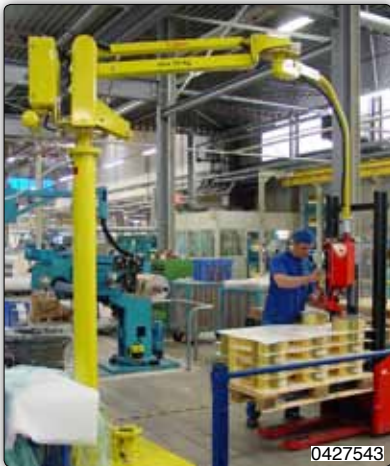
Manipulator with suction cups tooling for gripping and 90° manual inclination of little rolls. Vacuum is generated by a multi-stage "Venturi" type ejector.
