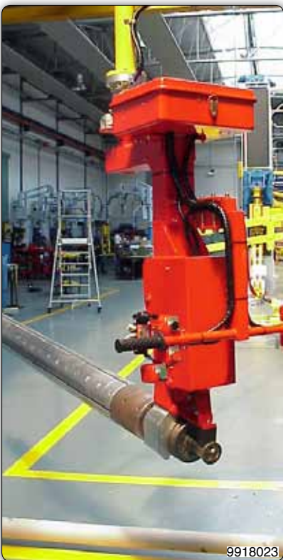
PMC type Partner manipulators, column mounted, complete with pneumatic gripper for picking and handling reel-carrier shafts.
