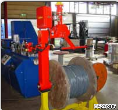
Gripping tooling with pin for handling and winding rolls.
