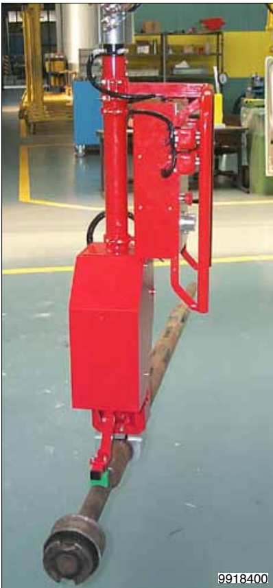
Manipulator complete with pneumatic gripper for picking and handling carrier shafts.
