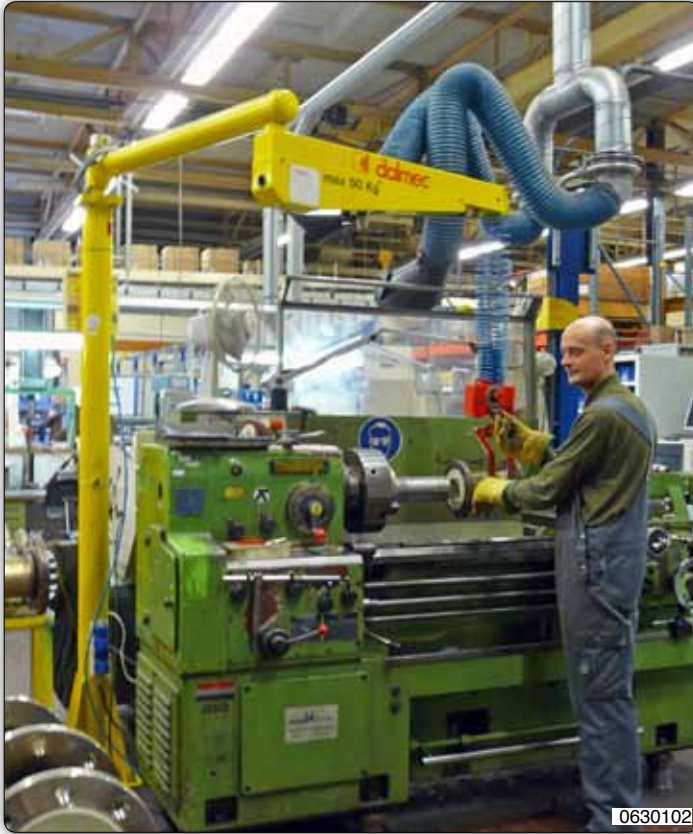
PVC type Posivel manipulator, column mounted, used to move mechanical components.
