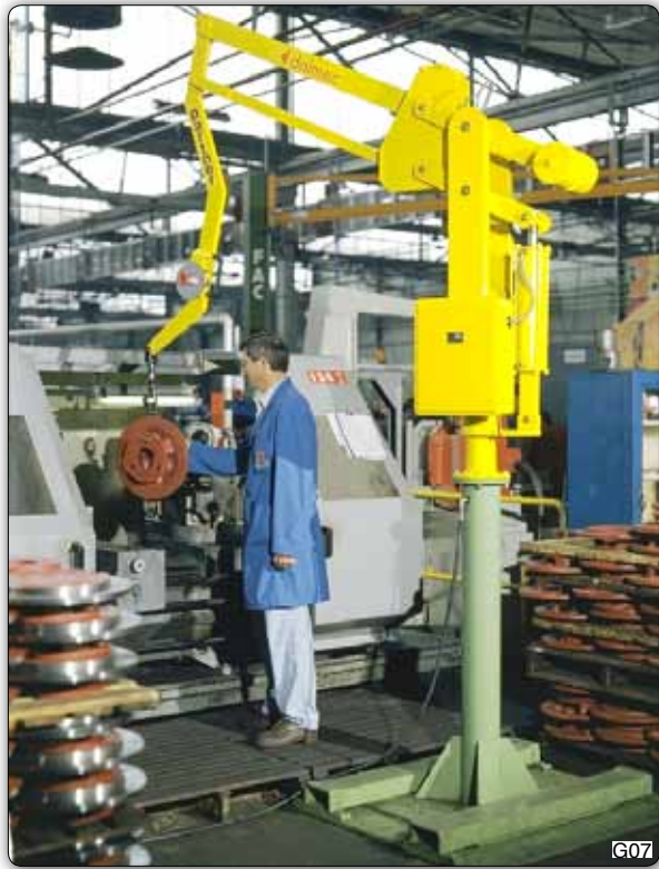
PSC type Partner manipulator, column mounted with gooseneck terminal arm, used to move epicycloidal spiders.
