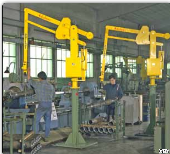
PSC type Partner manipulators, column mounted, used to position hydraulic cylinder barrels onto machine tools.
