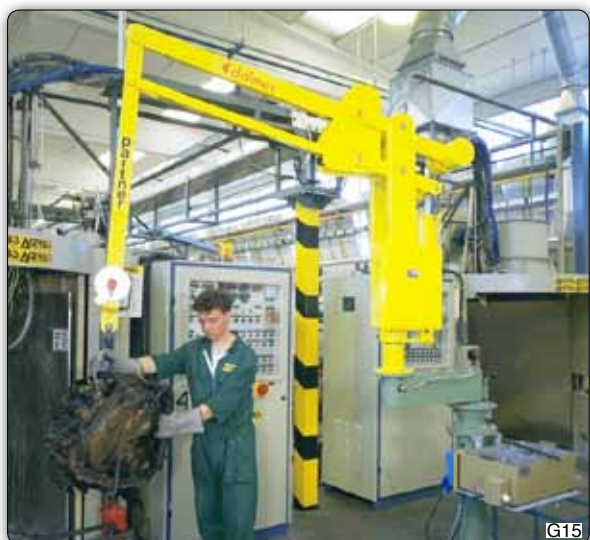
PSC type Partner manipulator, off-set column design, used to move dies for resin products.
