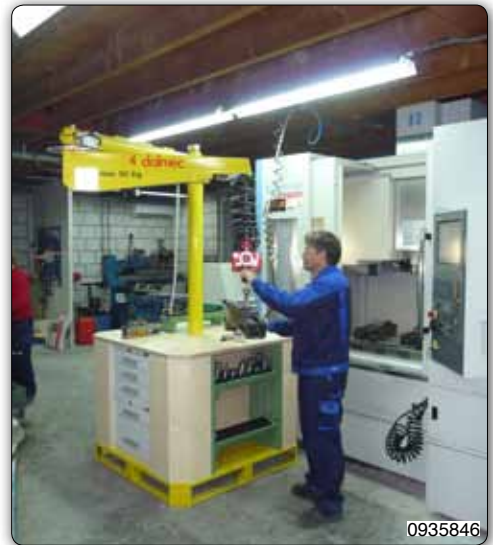
PVC type Posivel manipulator, column mounted, used to move mechanical components.
