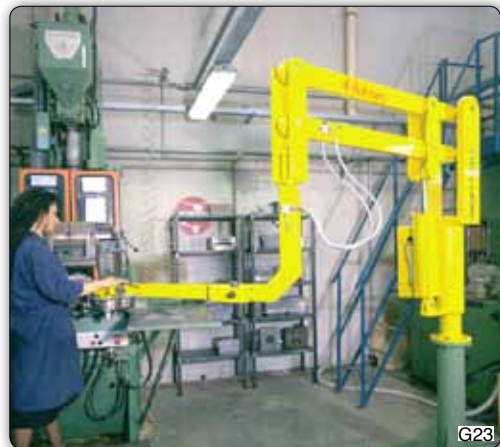
PMC type Partner manipulator, with low column and reach-in arm, and fitted with a device for handling moulds.
