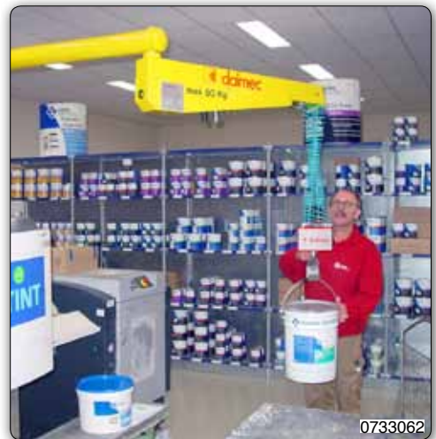
PVC type Posivel manipulator, column mounted, equipped with a hook for handling pails.
