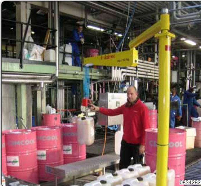
PVC type Posivel manipulator, column mounted, used to handle jerry cans.
