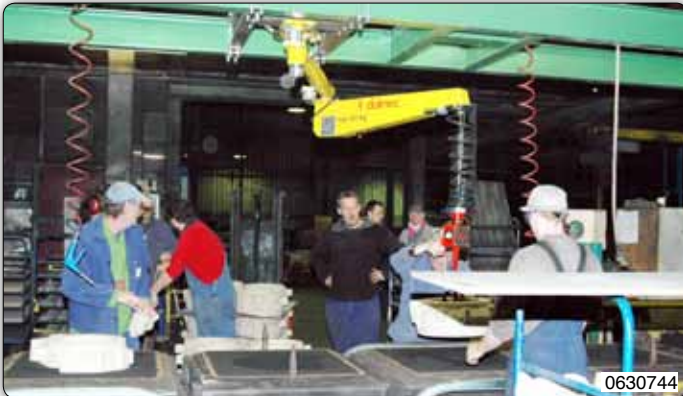
PVS type Posivel manipulator, overhead trolley mounted version, equipped with gripper picking system for moving core boxes. 0630744
