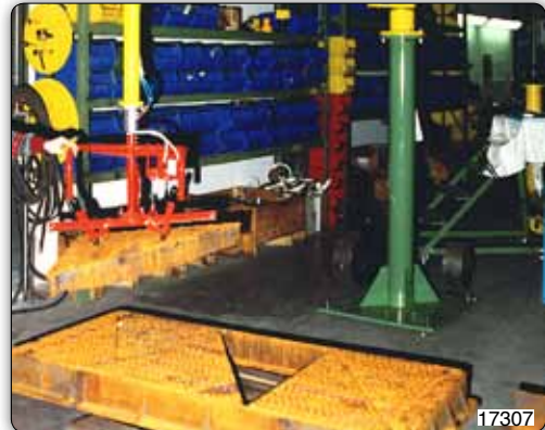
PMC type Partner manipulator, column mounted version, equipped with tooling for handling cast-iron covers. 17307
