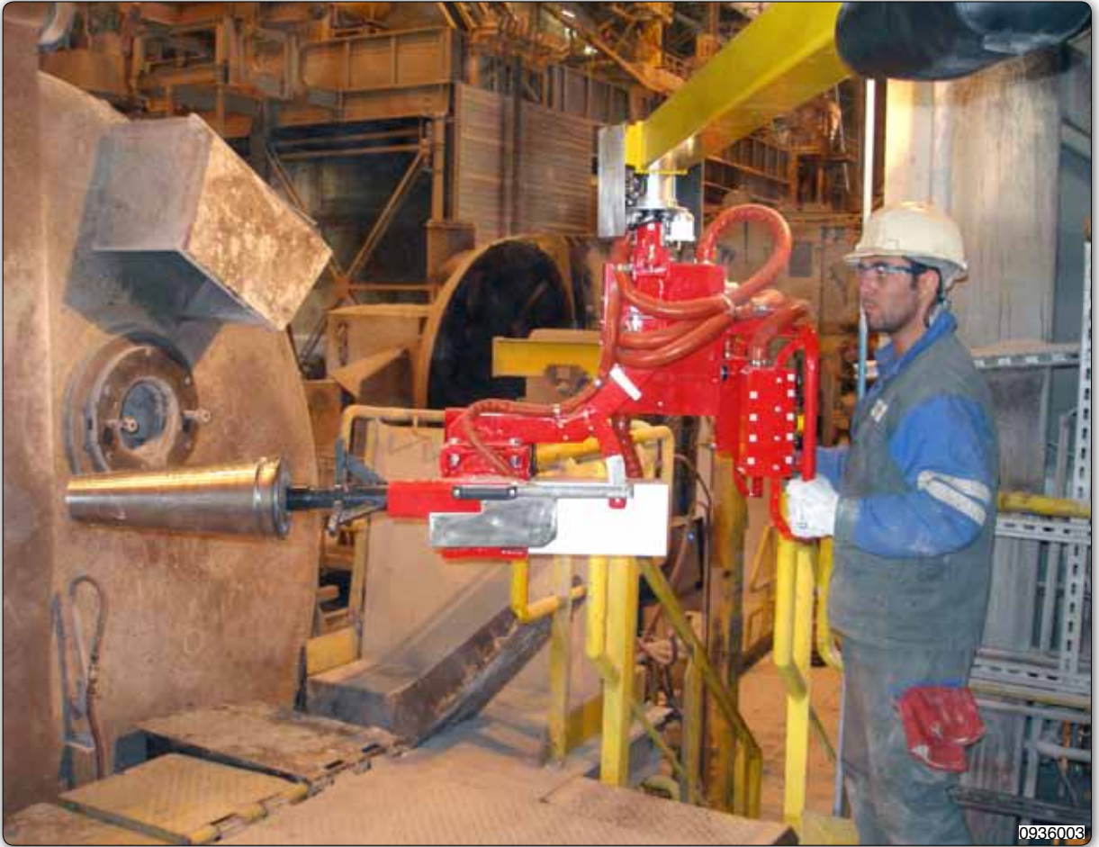
PMC type Partner manipulator, column mounted version, equipped with pneumatic gripper for castings.
