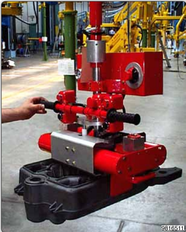
Manipulator equipped with a pneumatic gripper tooling for picking and handling parts of boilers.
