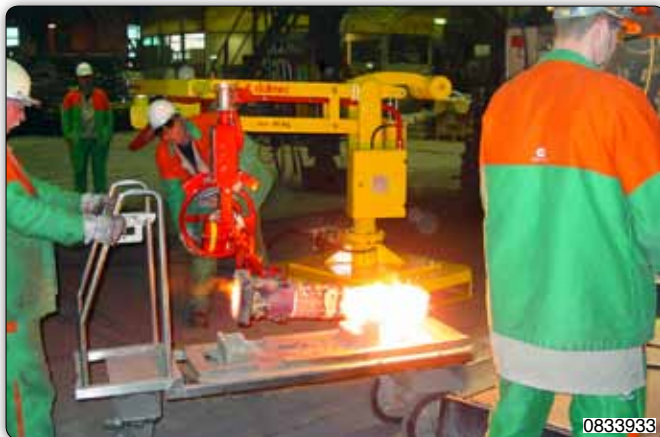
PMC type Partner manipulator, column mounted version, equipped with gripping jaws for moving incandescent parts.
