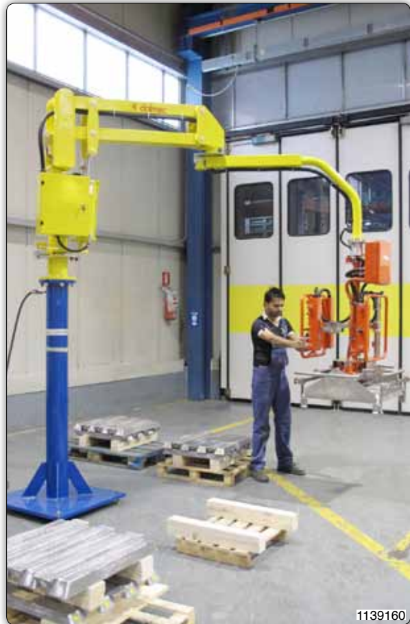
Manipulator with gripping jaws for picking and handling melted ingots.
