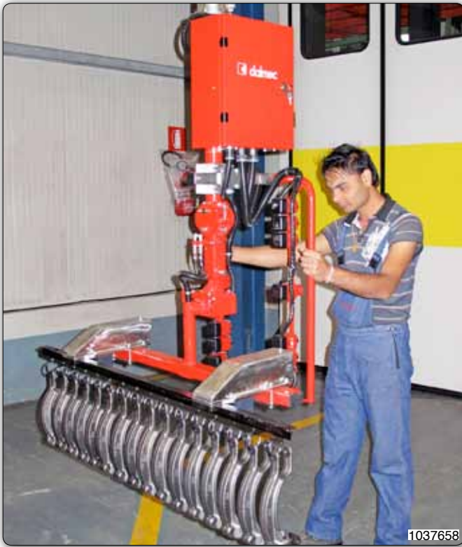
PMC type Partner manipulator, column mounted version, with tooling for handling castings.
