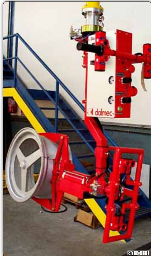
Manipulator with tooling for picking alloy rings, with manual rotation. 9816111
