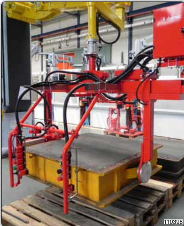
PMC type Partner manipulator, column mounted version, equipped with gripper picking system for moving cores.
