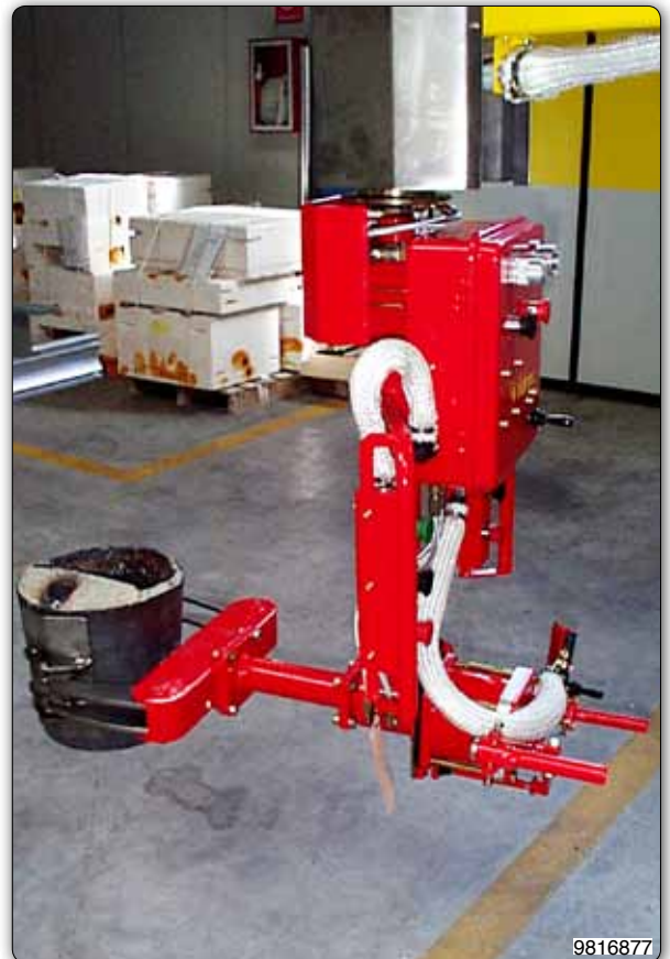
Manipulator with pneumatic gripping jaws for picking and emptying ladles.
