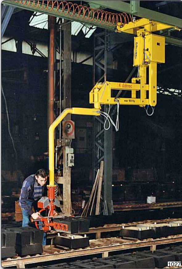
PMS type Partner manipulator, overhead trolley mounted version, with pneumatic jaws for picking casting dies.
