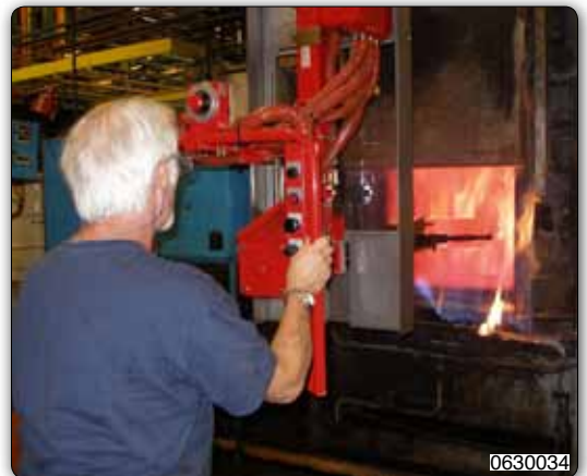
PMC type Partner manipulator, column mounted version, equipped with gripping jaws for moving incandescent parts.
