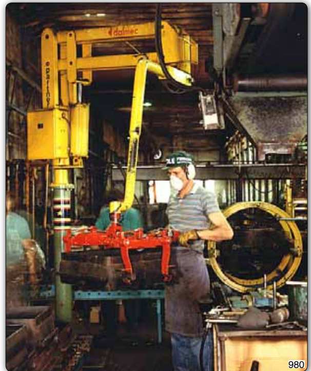
PMC type Partner manipulator, column mounted version, equipped with gripper picking system for moving cores.
