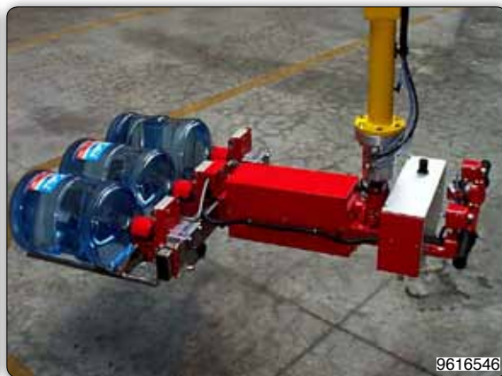
Gripping systems for gripping and handling of beverage containers with rotation/inclination of the load.
