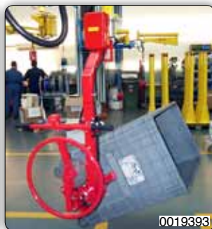
Gripping devices for handling containers of food products. In particular:
