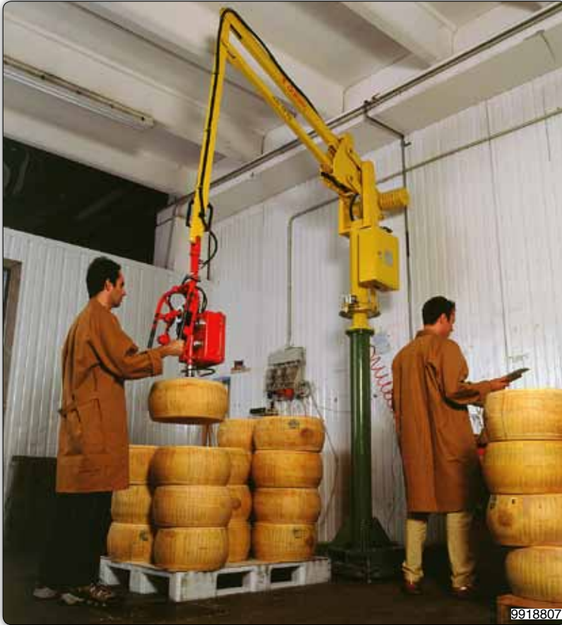
PSC type Partner Manipulator, column mounted, equipped with a suction cup tool for handling cheese in the cleaning area.
