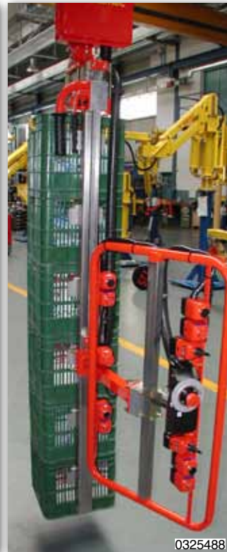
Partner Manipulator overhead trolley mounted version with pneumatic motorization, equipped with multiple adjustable hooks gripping system for handling 1 to 8 beverage crates having different dimensions.
