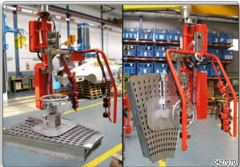
Suction cup tooling for gripping, pneumatic inclination and manual rotation of ice-cream moulds.
