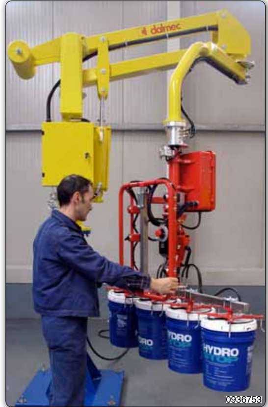
PMC type Partner manipulator, column mounted, for handling one or more pairs at once and handling from the packaging line to a pallet.
