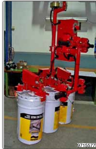
Pneumatic tooling head for handling three drums at the same time.
