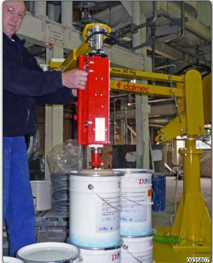
MIC type Microparter manipulator equipped with venturi vacuum system for gripping and handling drums.
