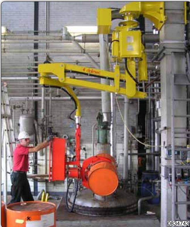
PMF type Partner manipulator, fixed overhead, made for picking and emptying drums, weighing up to 400 Kg.
