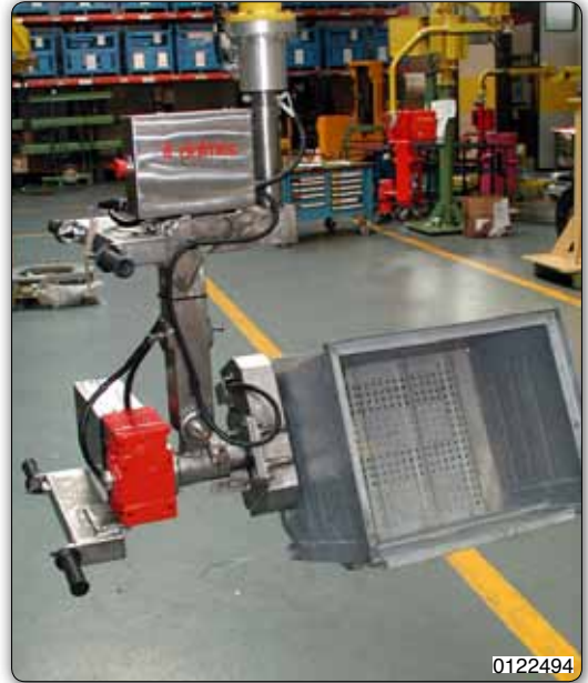
Manipulator with particular pinch jaws tooling, made of stainless steel for handling containers.
