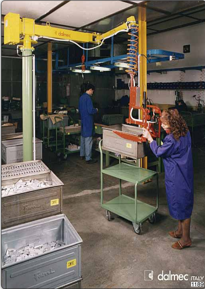
Posifil PFC column mounted Manipulator with forks tooling for handling crates.
