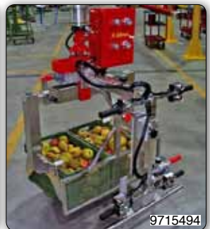
Partner Manipulator overhead trolley mounted version with pneumatic motorization, equipped with multiple adjustable hooks gripping system for handling 1 to 8 beverage crates having different dimensions.
