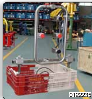
Partner Manipulator overhead trolley mounted version with pneumatic motorization, equipped with multiple adjustable hooks gripping system for handling 1 to 8 beverage crates having different dimensions.
