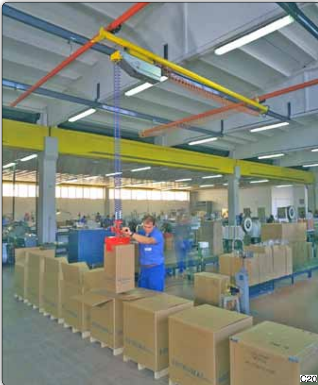
MPS type Minipartner manipulator, overhead trolley mounted, equipped with pneumatic jaws for gripping and handling boxes of different dimensions and weights. The tooling is fitted with a proportional valve to allow the operator to easily set the balancing system. The overhead trolley and downshop tracking system are made by Dalmec.
