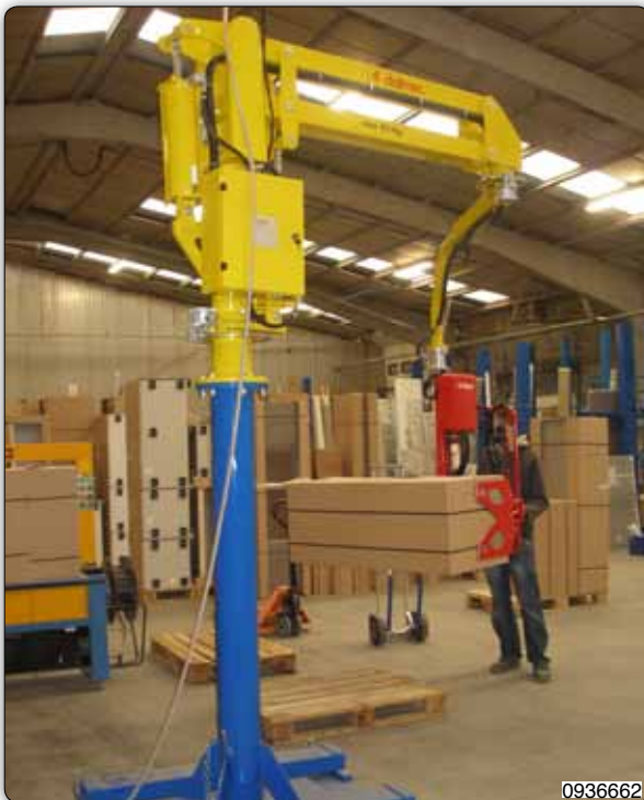
PMC type Partner manipulator, column mounted, fitted with pneumatic gripper tooling. The special design of the tooling jaws allows the user to grip and handle a particularly wide range of packaging.
