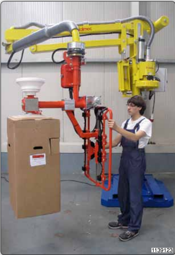
PMC type Partner manipulator, column mounted on portable baseplate, equipped with double suction cups gripping system for gripping industrial lamps and their packaging.
