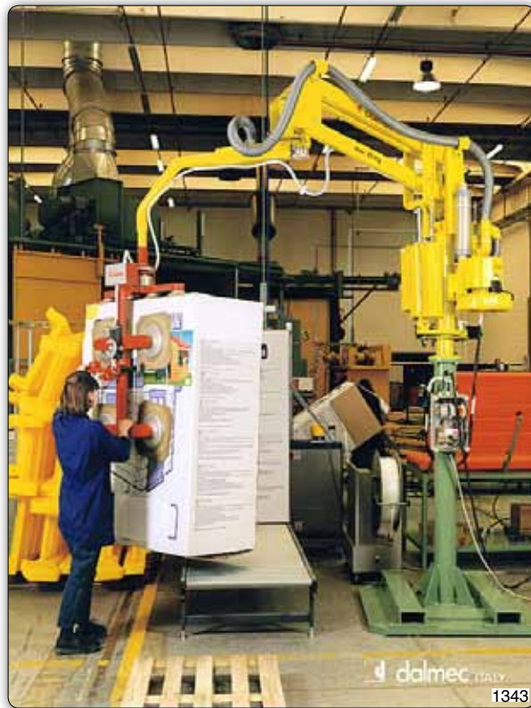
PMC type Partner manipulator, column mounted, fitted with suction tooling to grip and handle cardboard boxes from a packaging line to a pallet.
