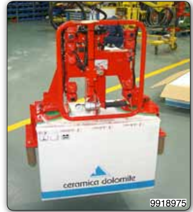
PFC type "Posifil" manipulator, column design, equipped with gripper system for picking sanitary ware, inserting it in cardboard boxes, picking the packed boxes and putting them on to pallets.
