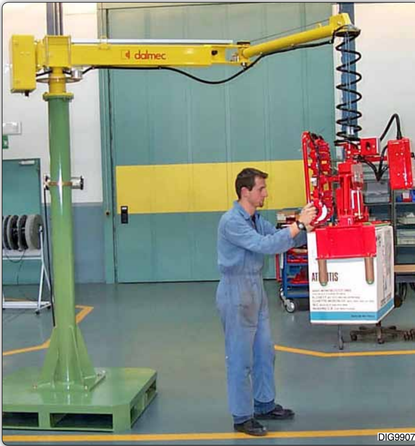
PFC type "Posifil" manipulator, column design, equipped with gripper system for picking sanitary ware, inserting it in cardboard boxes, picking the packed boxes and putting them on to pallets.
