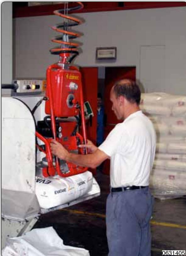
Posifil manipulator, column design, used to handle bags from the pallet to the hopper. Vacuum is generated by a multi-stage "Venturi" type ejector.
