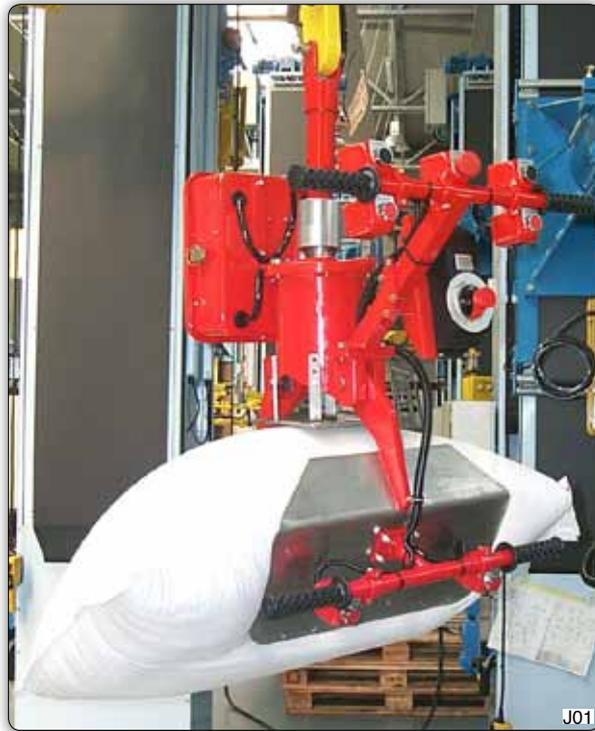
Manipulator with pneumatically actuated gripper picking system.
