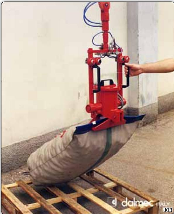
Manipulator with pneumatic clamping grippers which allows the bags to be inclined from the horizontal to the vertical and vice versa.
