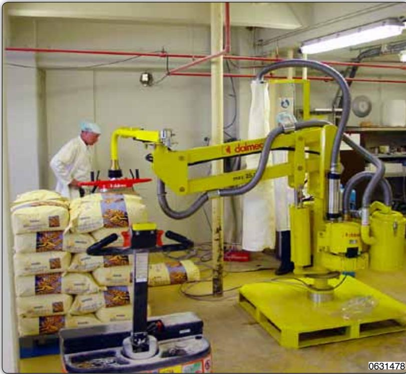
PMC type Partner manipulator, column design, special low profile unit, to enable to operate in a room with low ceiling. The equipment allows the bags to be picked from a pallet and to be loaded onto a hopper.
