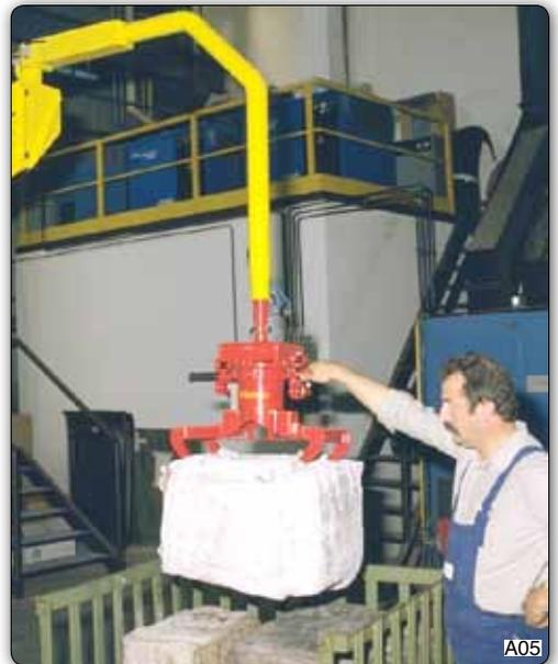
Manipulator with pneumatically actuated grippers, which hold the bale by gripping into the product itself.
