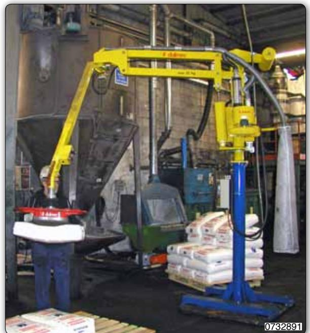
PMC type Partner manipulator, column mounted, equipped with suction head to pick bags from a pallet and loading them to a mixer.
