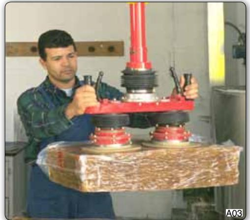
Tooling head for handling rubber bales with independently swivelling suction cups.
