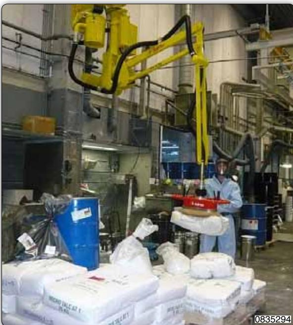
PSS type Partner manipulator, overhead trolley mounted version in Dalmec track. The operator picks bags from various pallets in the "picking" area and deposits them to a common pallet.
