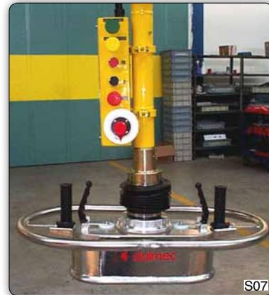
Suction device made of stainless steel.
