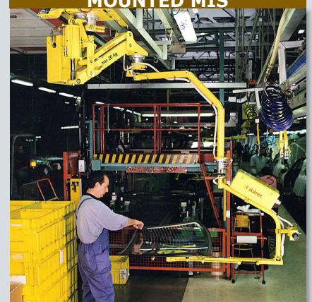
OVERHEAD TROLLEY MOUNTED MIS
