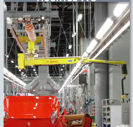
OVERHEAD TROLLEY MOUNTED PFS
