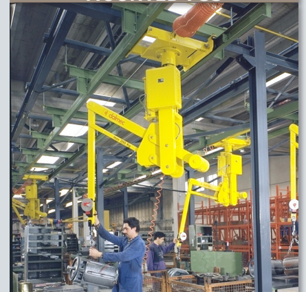
OVERHEAD TROLLEY MOUNTED PSS
